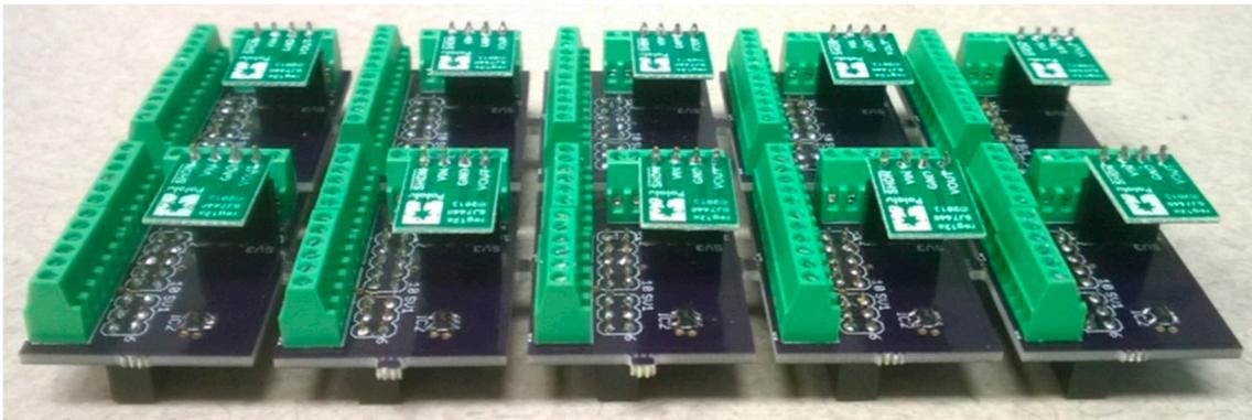
**Figure 2.** Custom sensor boards for TelosB motes.
