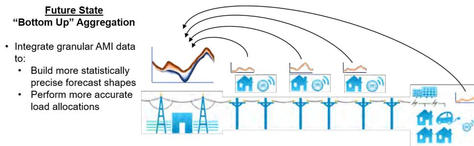
Figure 13: Illustration of Using a Bottom up Aggregation for Future System Planning Studies.
