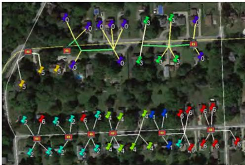
(e) Result of K-means clustering algorithm using Voltage and GIS information.
