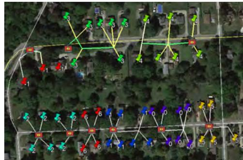
(f) Result of DBSCAN clustering algorithm using Voltage and GIS information.
