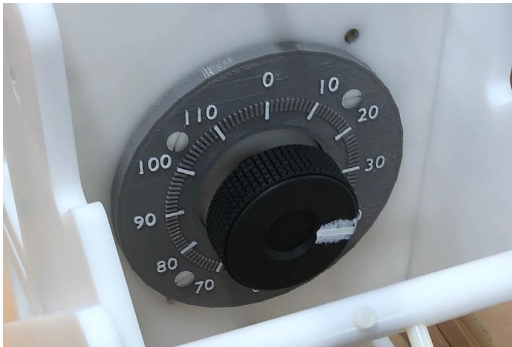
Figure 12: Adjustable knob that is set at half the patient's body weight.
