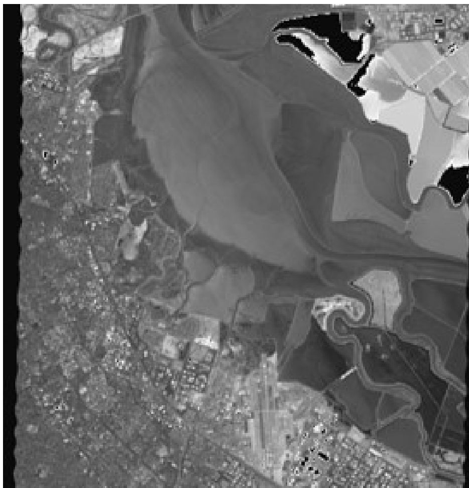
Figure 10: CNN-JPEG compressed spectral band without reconstruction
