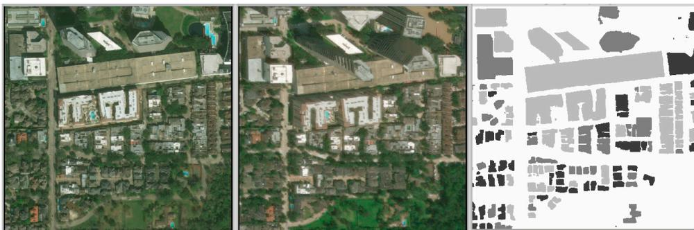
**Figure 2.** From left to right: The before-disaster, after-disaster, and damage magnitude inference images from our pipeline.
