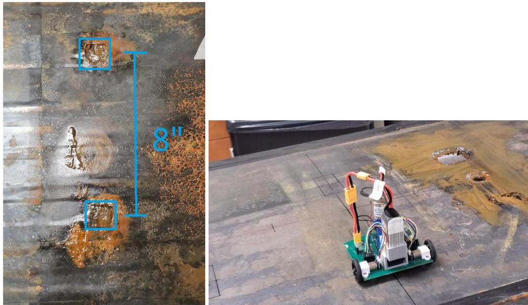
**Figure 27 - A picture of the underside of the plate. The two corroded sections are outline in blue, and the robot drove on the opposite of the pictured side. Also included is a picture of the robot driving on the uncorroded side.**
