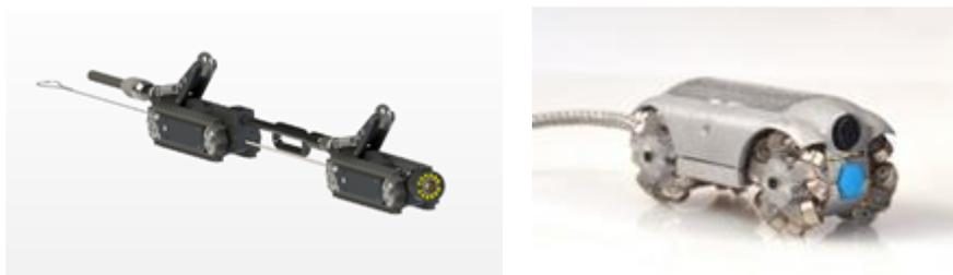
**Figure 3 - On the left, a pipe robot meant for 4” pipes designed by Versatrax [8]. On the right, a pipe robot meant for 2” pipes designed by Honeybee [9].**
