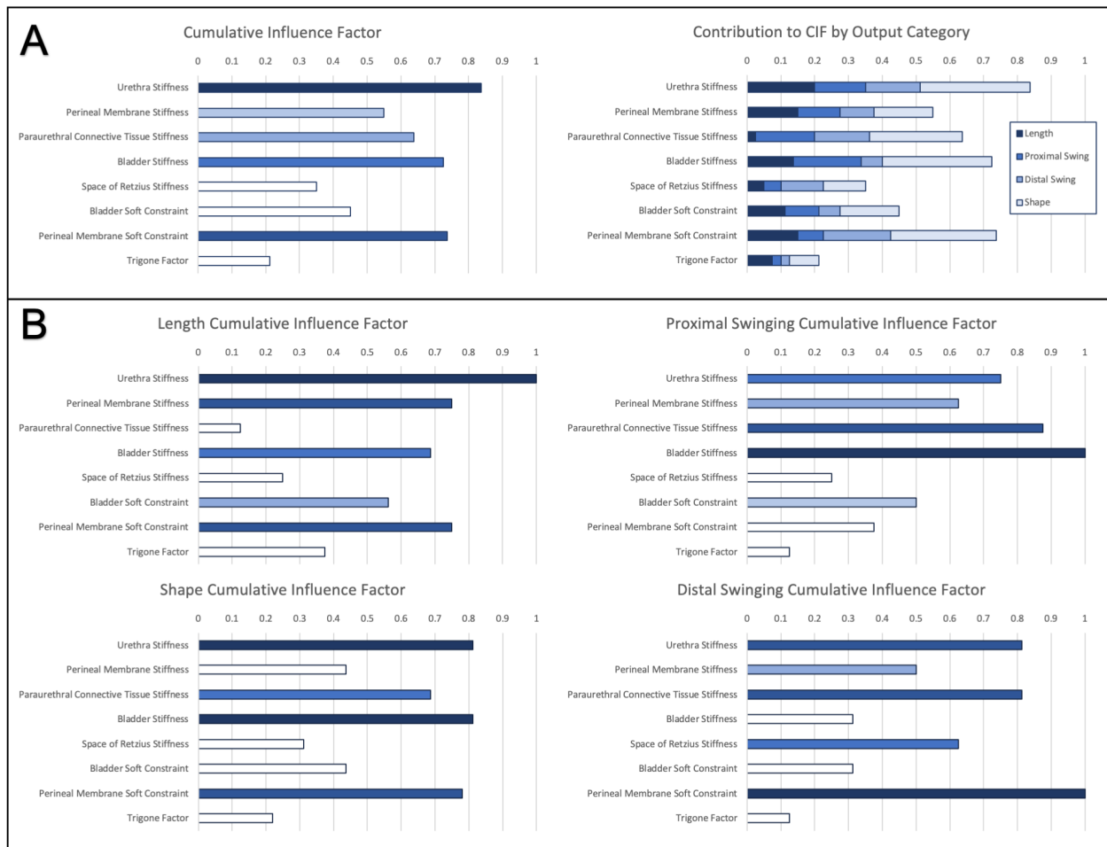
Figure 3.10: Graphs of the final Latin hypercube sampling–partial rank correlation coefficient results—the cumulative influence factors (CIFs). A) Displays the overall CIF for each input variable. The darkest color indicates the overall most influential input and the lightest the overall least influential input, while white bars indicate variables that did not reach meaningful influence (CIF \geq 0.5 ). On the right, the CIFs are broken down by output variable category. B) Displays the CIFs as if the output variables within each output category were considered individually, demonstrating how an input variable’s influence may change with the choice of output variables. The bars are color coded using the same convention as that of the overall CIF graph [166]. This figure was reprinted by permission from The International Urogynecological Association: Springer; International Urogynecology Journal; Megan R Routzong, Liam C Martin, Ghazaleh Rostamina, and Steven D Abramowitch. Urethral support in female urinary continence part 2: a computational, biomechanical analysis of Valsalva. International Urogynecology Journal , 2021; © 2021 The International Urogynecological Association.
