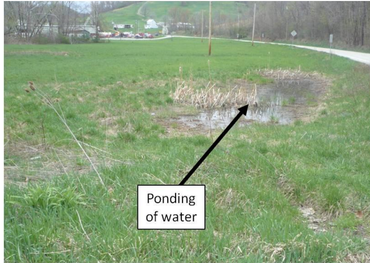
Figure VII-5 - Ground settlement over a longwall panel allowed water to pond in depression (Photograph courtesy of N. Iannacchione).
