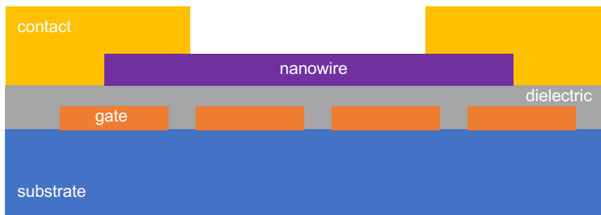
Figure 3.3: Schematic sideview of a two-terminal nanowire device on local electrostatic gates.
