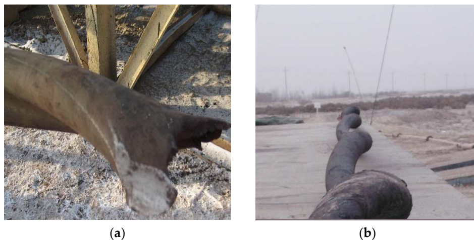
Figure 1. Tubing damage caused by perforating shock loads: (a) tubing breaking; (b) tube buckling.
