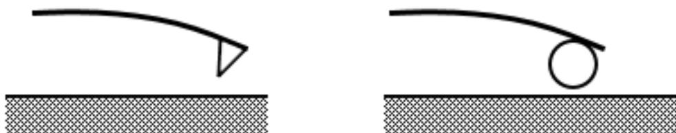
**Figure 6 Schematic representation on an adhesion test using a standard AFM tip (LEFT) and a colloidal probe tip (RIGHT)**
