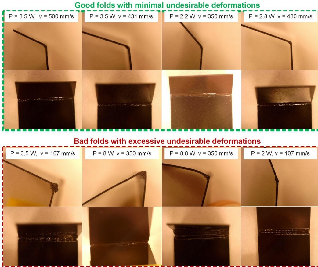
Figure 57: Side view and top view images indicating the influence of laser conditions on fold distortion and quality , where too much heating leads to excessive deformation manifested as highly distorted hinges. ( P = 3.5 W, v = 500 mm/s, 2wx = 1 mm, n = 9 ) and ( P = 3.5 W, v = 107 mm/s, 2wx = 1 mm, n = 9 ) were imaged using SEM as well.
