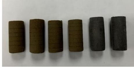
**Figure 3.1** -Photos of the sandstone and slate samples (the slate samples are the two at the rightmost side of the picture).
