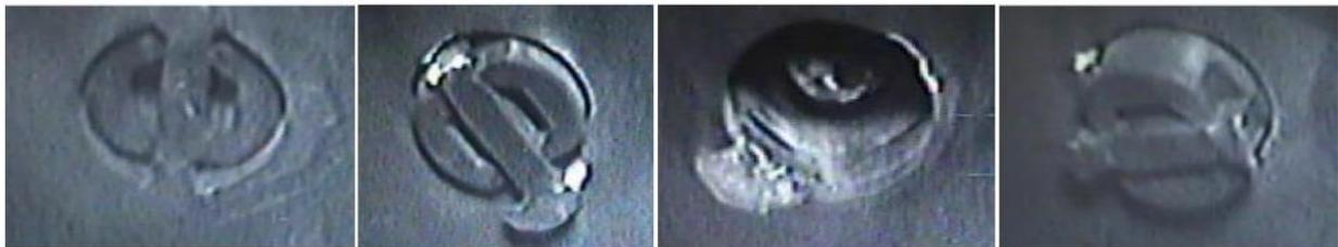
**Figure 7.** Intact Baffle-former Bolt (Left) and Failed Type 347 Baffle-former Bolts in a U.S. 4-loop Downflow PWR
