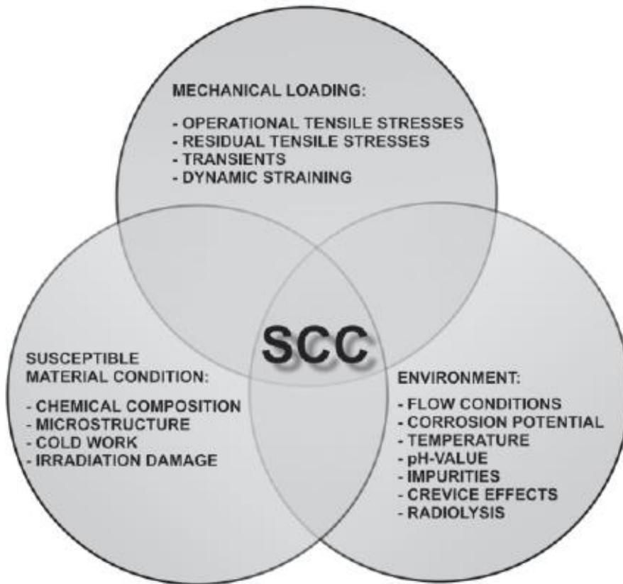
**Figure 8.** Elements of Stress Corrosion Cracking - Adapted from Reference 8
