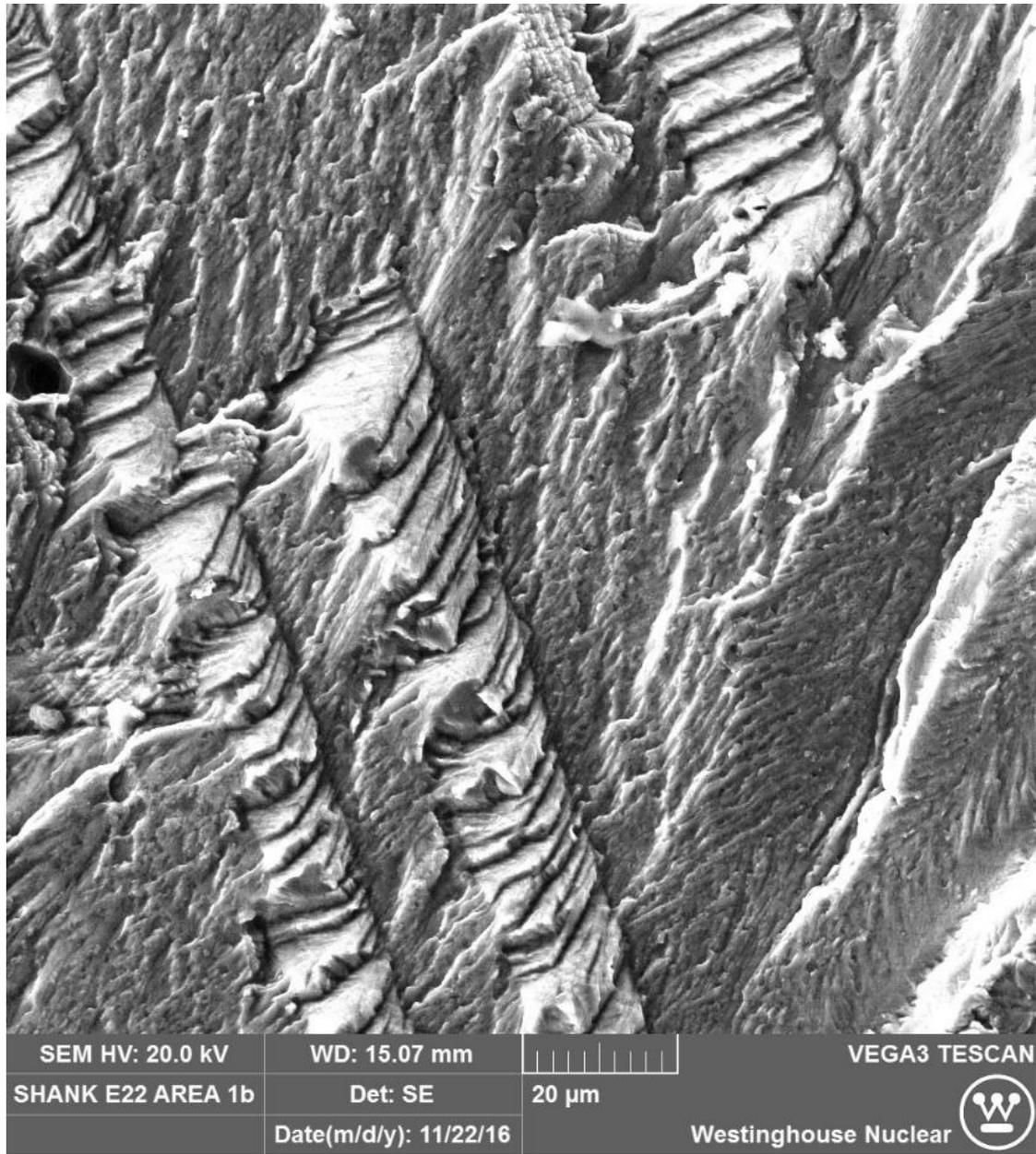
**Figure 33.** TG Cracking with Slip Bands in Bolt E22
