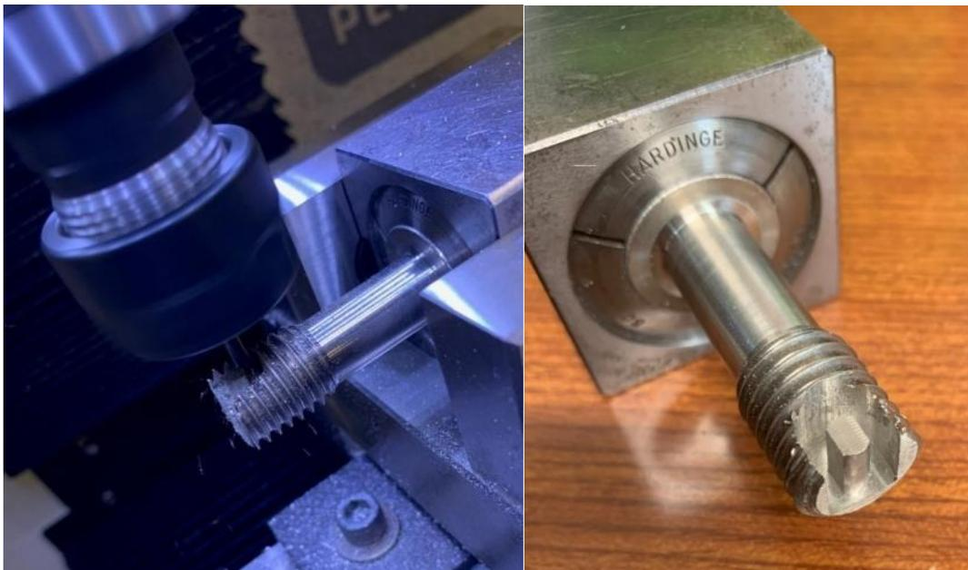
**Figure 63.** Machining of 4-point bend samples from unirradiated practice bolt
