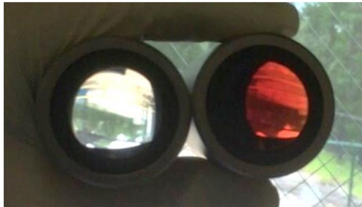
**Figure 20.** New lens (left) compared to lens used for baffle-former bolt examination (right)
