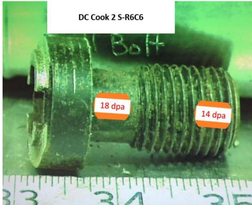
**Figure 65.** Approximate locations for specimen machining for DC Cook 2 S-R6C6
