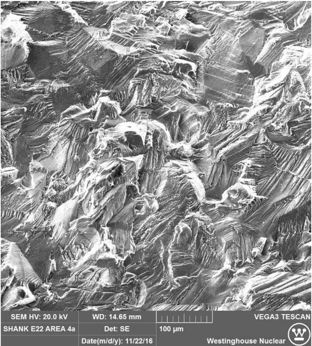
**Figure 32.** TG Cracking in Bolt E22 Feathery cracking with slip bands, limited secondary cracking, no striations
