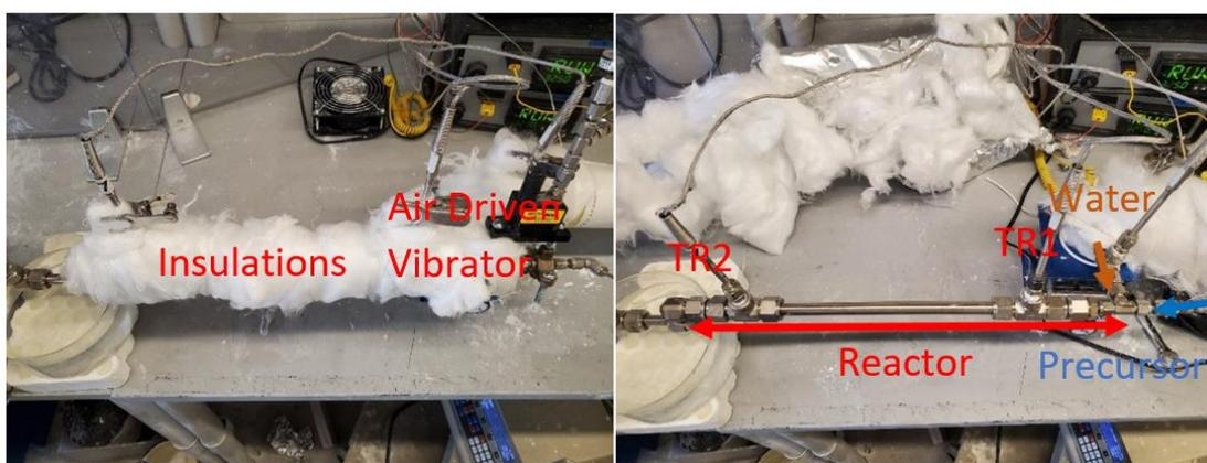
Figure S 2. Photo showing (a) reactor ready for running synthesis, (b) the reactor after removing the insulations and the vibrator. The reactor length is defined as the distance from the midpoint in the T mixer to the end of the tubular reactor as shown in the picture.
