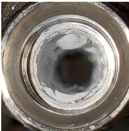
**Figure 15. A photo showing the fouling observed in a  $\frac{1}{2}$ ” tubular reactor after a synthesis at  $\sim 280$  C for 20 mins.**
