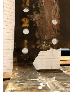
d) bearing region following testing and removal of stiffeners
