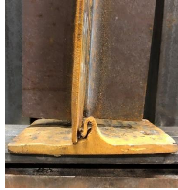
c) complete collapse of the web
