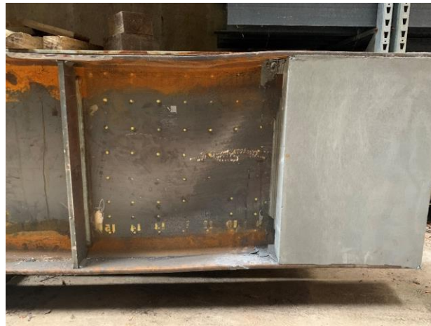
c) observed web buckling behaviour (image mirrored)
