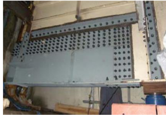
b) bolted beam end replacement (Wakabayashi et al. 2013)
