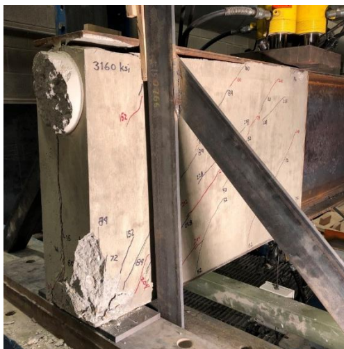
c) concrete bearing failure
