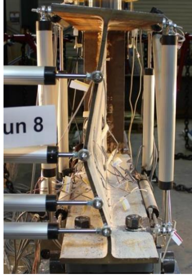
d) crippling of undamaged web
