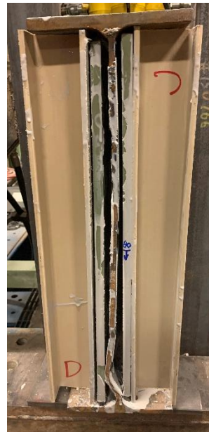
c) catastrophic debonding at V = 81.8 kips
