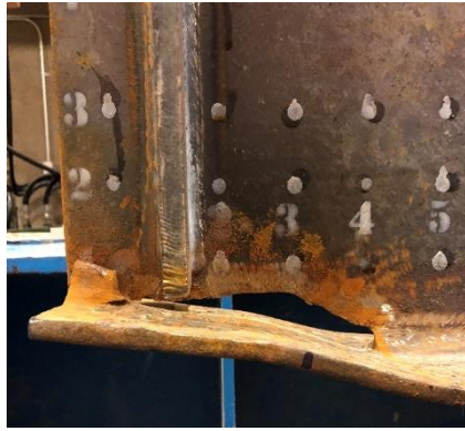
b) residual distortion of bearing region after testing
