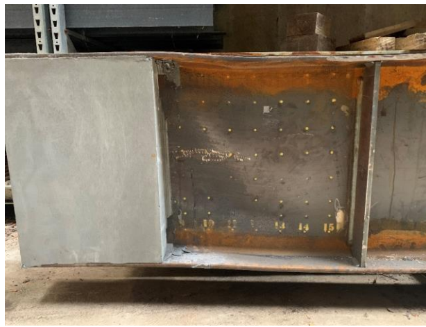
Figure 53 Girder 4B Following Testing Showing Well Controlled Panel Buckling
