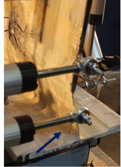
e) crippling of damaged web
