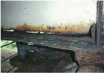
a) prototype corrosion damage
