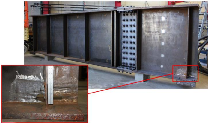
b) specimen with damaged end region
