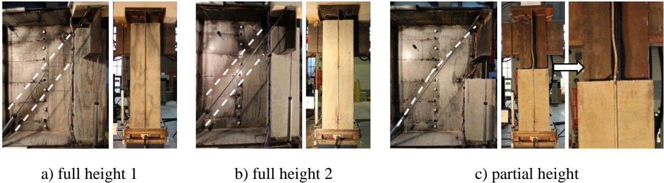
Figure 11 Failure Modes of UHPC Encased Girders Reported by McMullen and Zaghi (2020)
