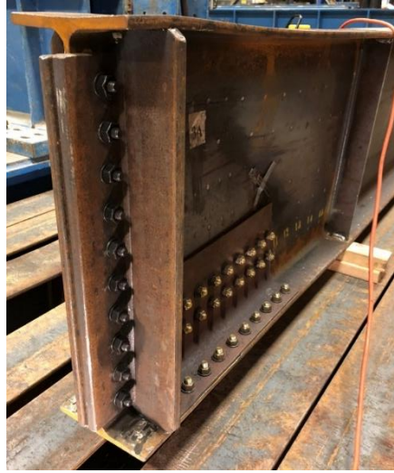
a) bearing region following testing
