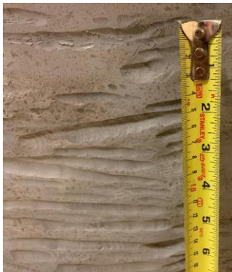
a) SSPC SP5 surface preparation
