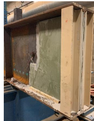
c) completed FRP repair
