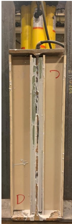
a) bearing at beginning of test
