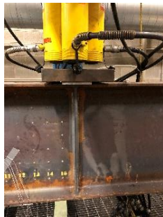
a) Monotonic Tests of Girder Ends A
