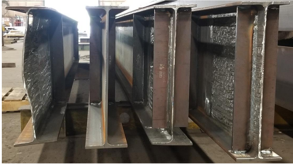
a) Girder 8; fabricated without a stiffener (not tested in this study) b) W24 x 55 prior to machining c) Girder 2 d) Girder 1
