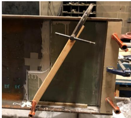
b) installation of FRP
