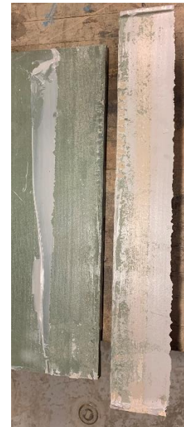
d) debonded surface of W3 and GFRP plate
