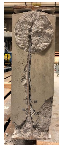
d) encased concrete mitigated further distortion of web (distortion seen was present at concrete placement); concrete intentionally removed to show web
