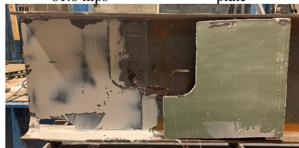
f) debonding of East side GFRP plate (affixed to smooth steel)
