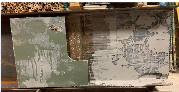
e) debonding of West side GFRP plate (affixed to 'corroded' steel)
