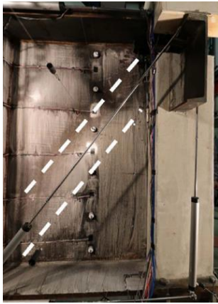
a) full height UHPC repair McMullen and Zaghi (2020)
