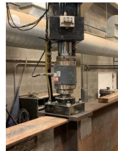
b) Fatigue Conditioning of Girder Ends B
