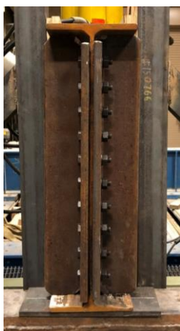
Figure 34 Bolted Steel Repair Detail for Girder 3
