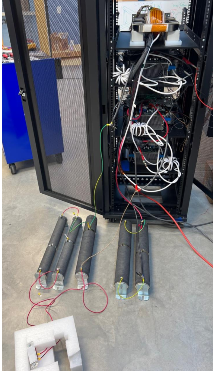
Figure 23:Resistive Load Setup for TAB Test Bed
