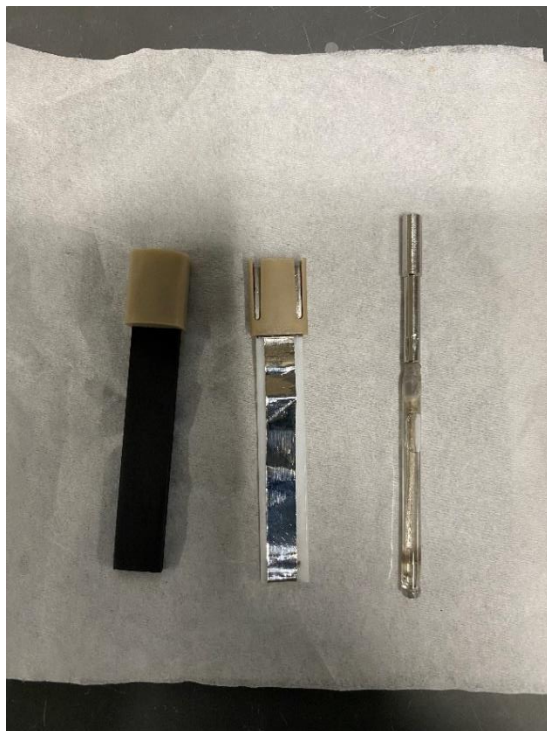
Figure 13. Electrodes that are Connected to the Vial Cap
