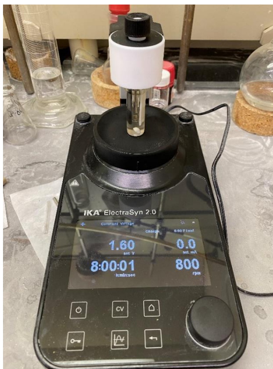
Figure 15. Example of an Electrochemical Reaction Setup on the Electrasyn 2.0
