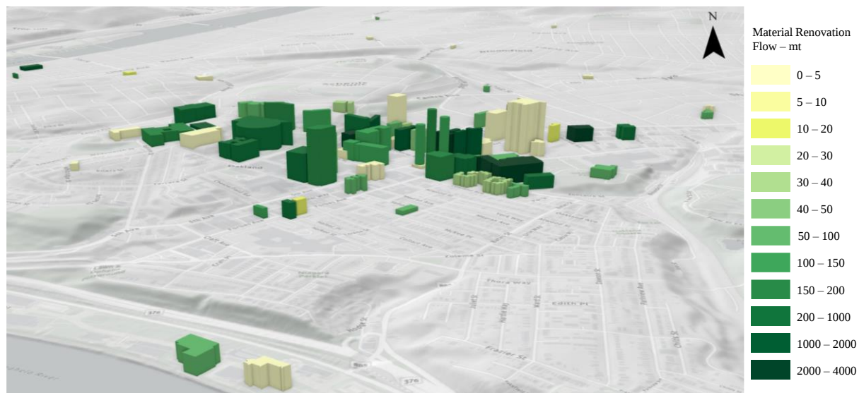
Figure 22 Spatial distribution of the total material renovation flow between 2020 and 2030 in the studied building stock. Note: mt= metric ton
