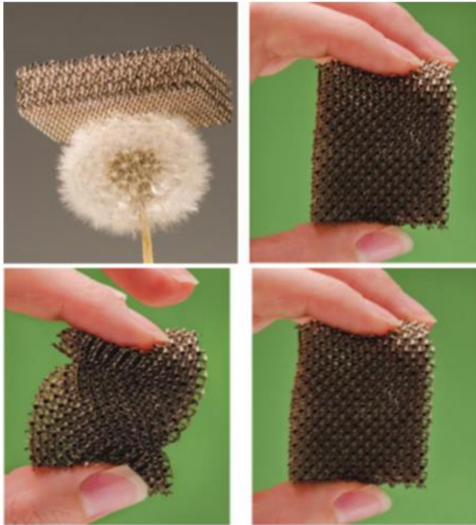
Figure 9 Ultra-light metamaterial demonstrating ultra-low density and excellent recoverability (Surjadi et al., 2019).
