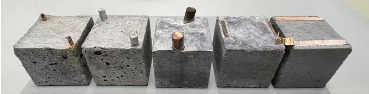
Figure 44 Two inches by two inches cement cubes added with Graphite powder and different electrodes for electrical resistance measurement.
