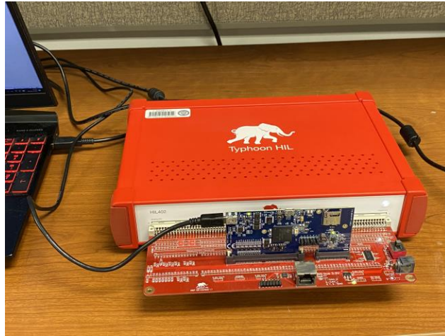
Figure 43: Experimental setup for the Control Hardware-in-the-Loop simulation
