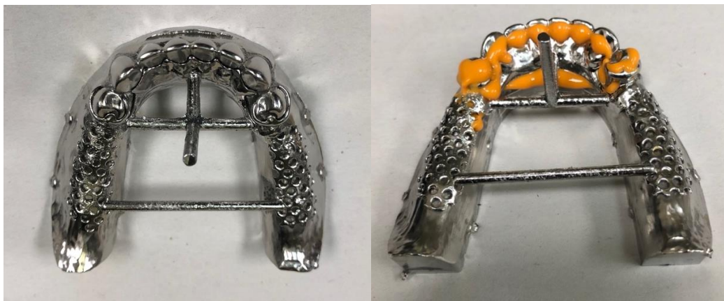
Figure 6A and 6B (A) SLA-Cast framework seated on the metal reference model (B) PVS fit testing of SLA-Cast framework seated on the metal reference model
