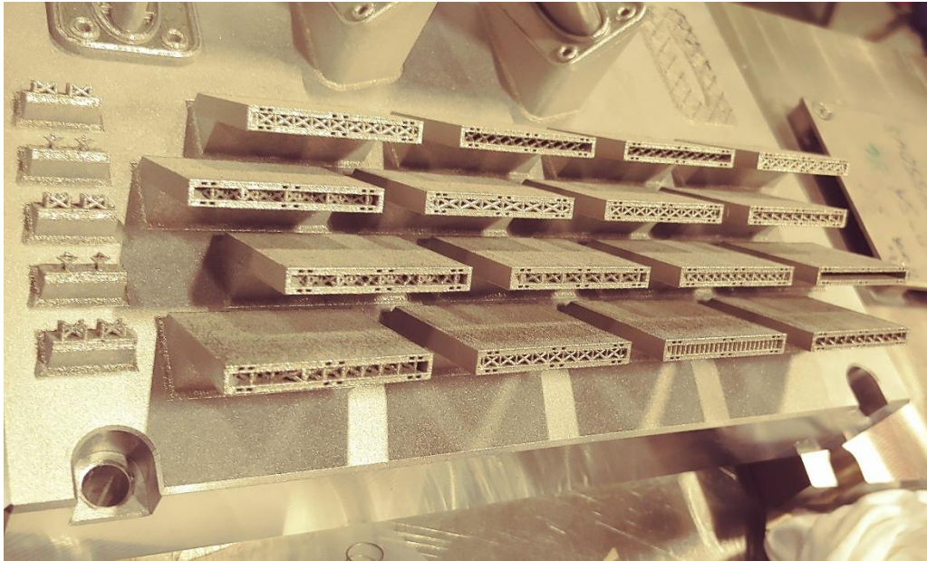
Figure 2.9 (Top) Cartoon depicting the 45° orientation, and (bottom) AM fabricated IN718 coupons on the build plate
