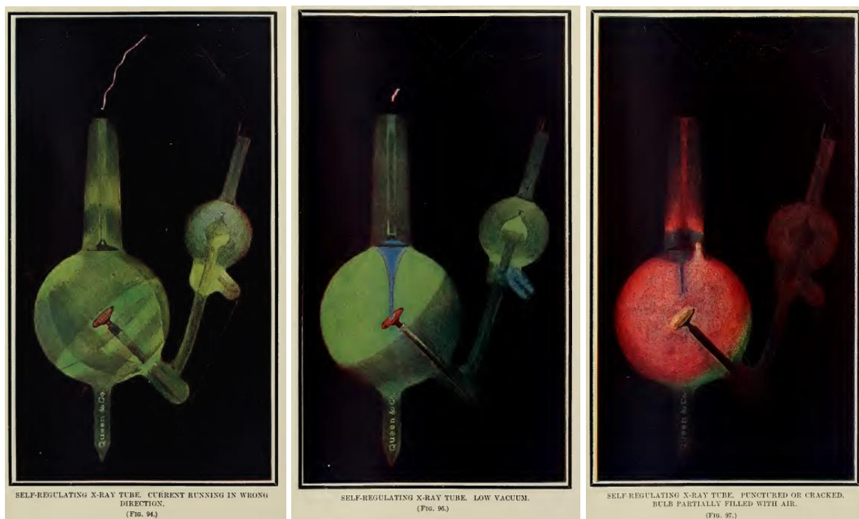
Figure 24: Plates from Kassabian (1910) showing, from left to right, a backward-running current producing illumination on the wrong side of the tube, low vacuum (i.e., high gas pressure) producing a blue light, and a cracked bulb.
