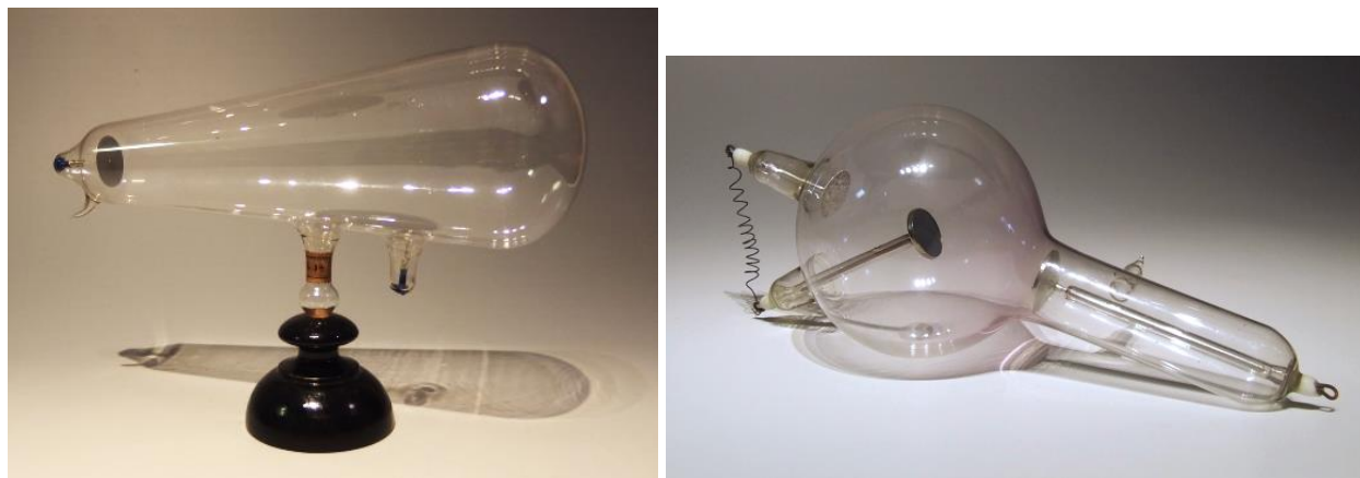
Figure 22: Left: a Crookes-Hittorf tube from 1896, with cathode is on the left side of the image. Right: a dual anode tube (c. 1910), with the central anode plane angled 45 degrees to the cathode. These were sometimes referred to as “focus tubes” with a concave cathode invented by Elihu Thomson to purportedly focus the rays onto a small point of the central anode. Images courtesy of Henk Dijkstra of the Cathode Ray Tube site.
