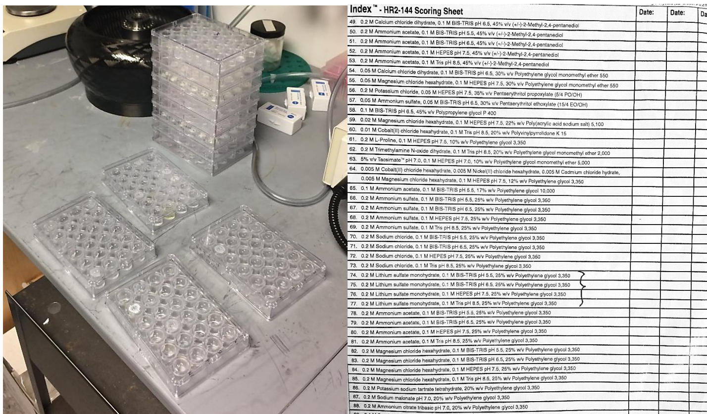
Figure 16: A collection of screening arrays (left). Each well contains different conditions as listed (right).
