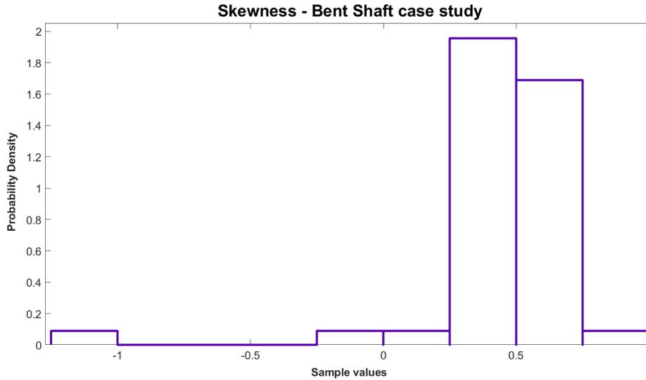
Figure 44: The skewness distribution for a bent shaft is an input for the Bayesian network.
