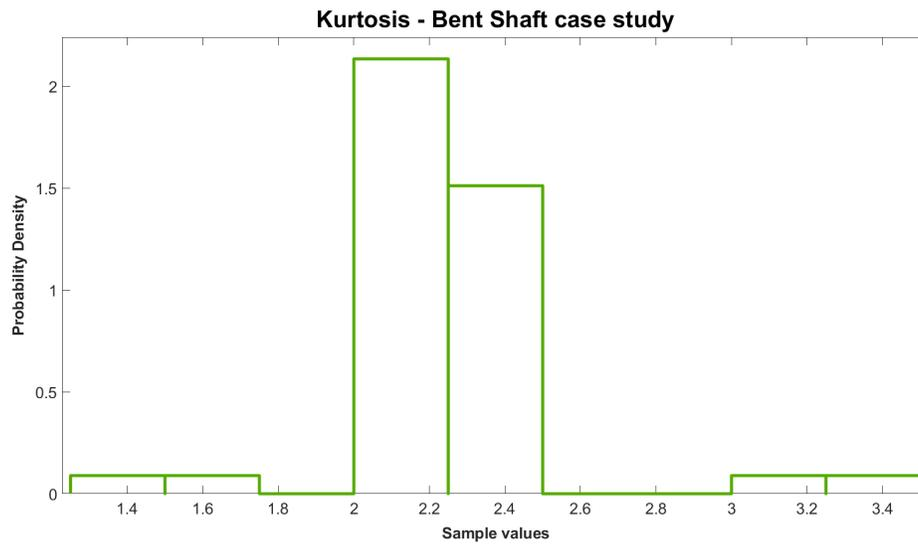
Figure 45: The kurtosis distribution for a bent shaft is an input for the Bayesian network.
