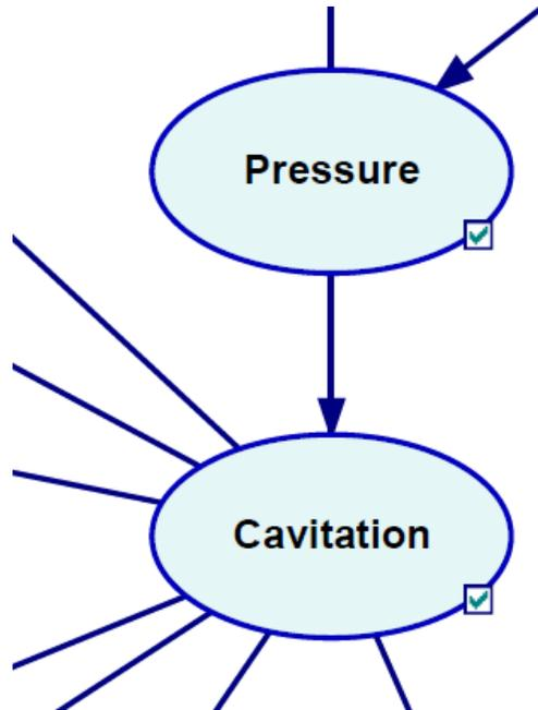
Figure 20: A change in suction pressure causes cavitation.
