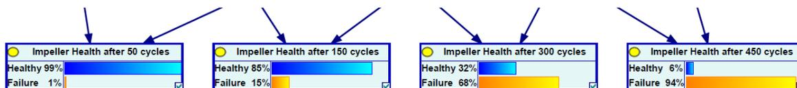
Figure 51: The pump is 94% likely to fail by 450 cycles due to a bent shaft.
