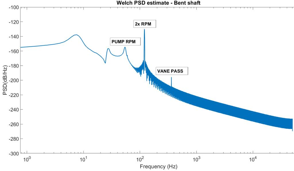
Figure 7: The vibration signal of the pump running with a bent shaft shows a high amplitude spike at  $2\times$  motor RPM.
