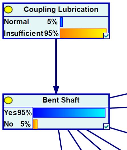
Figure 50: The likelihood of insufficient coupling lubrication is 95%.
