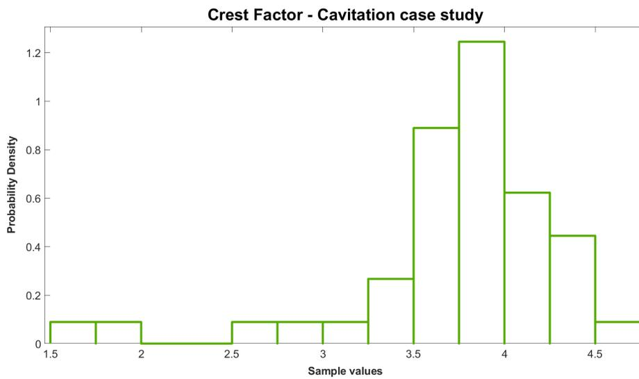
Figure 37: The crest factor distribution for cavitation is an input for the Bayesian network.
