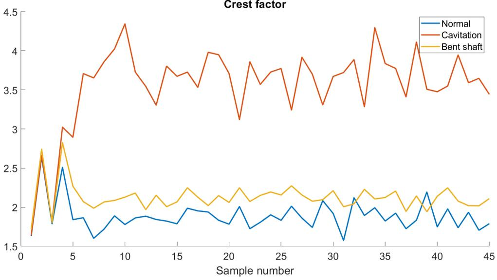
Figure 8: The crest factor values of the signal are distinct for cavitation.
