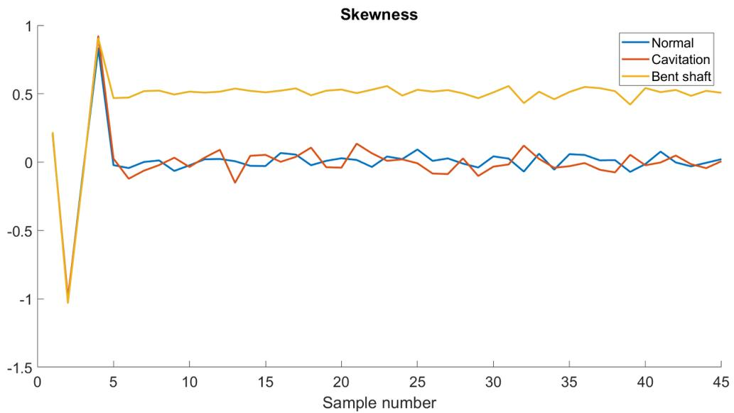
Figure 10: The skewness values of the signal are distinct for a bent shaft.
