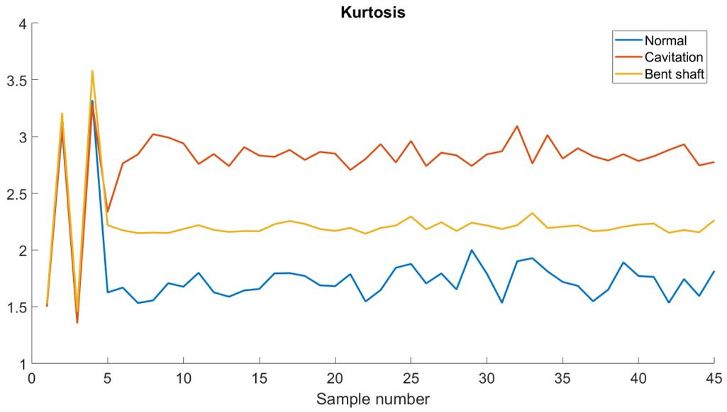
Figure 9: The kurtosis values of the signal are distinct for each of the three modes of operation.
