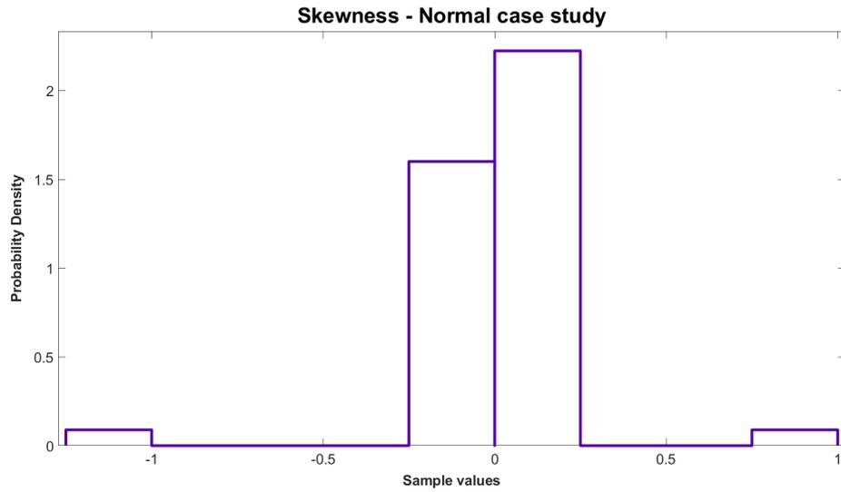
Figure 25: The skewness distribution for normal operation is an input for the Bayesian network.
