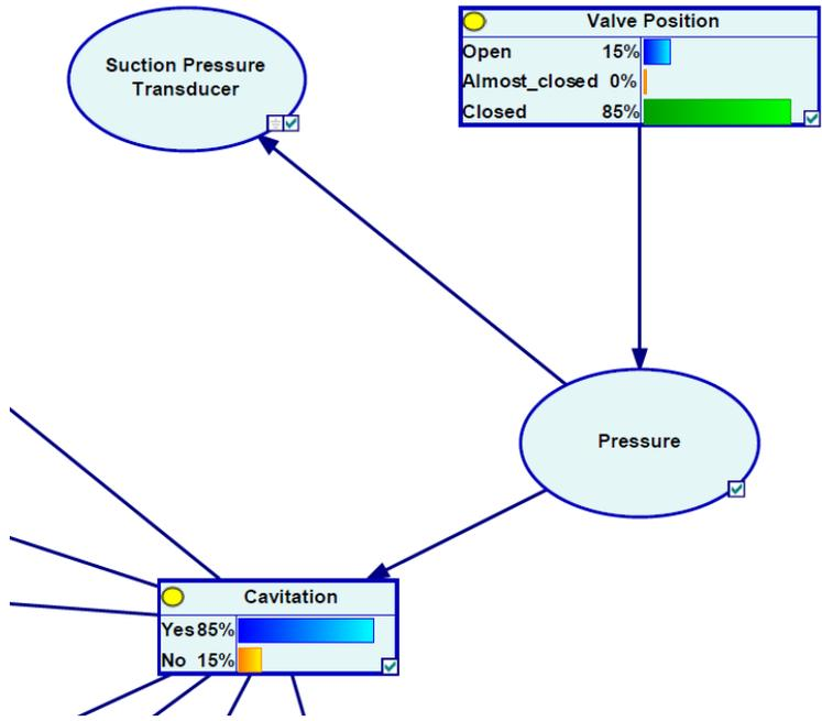
Figure 41: The likelihood of a malfunctioning valve is 85%.
