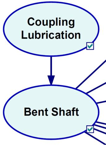
Figure 21: A bent shaft depends on the lubrication state of the coupling.
