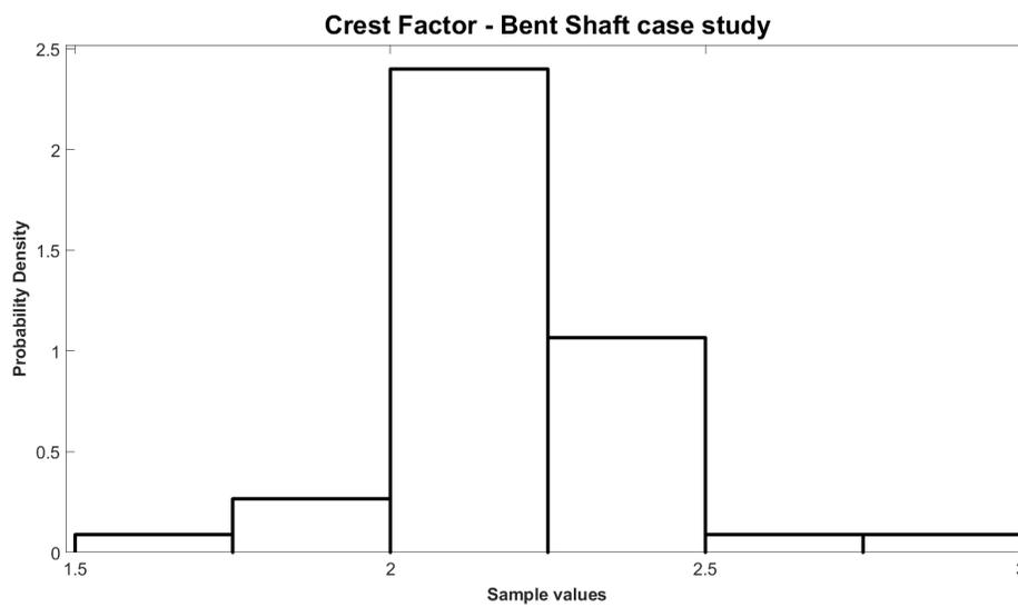
Figure 46: The crest factor distribution for a bent shaft is an input for the Bayesian network.
