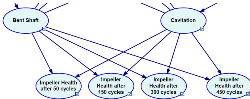
Figure 23: The remaining life of a pump changes conditional to the current diagnosis.
