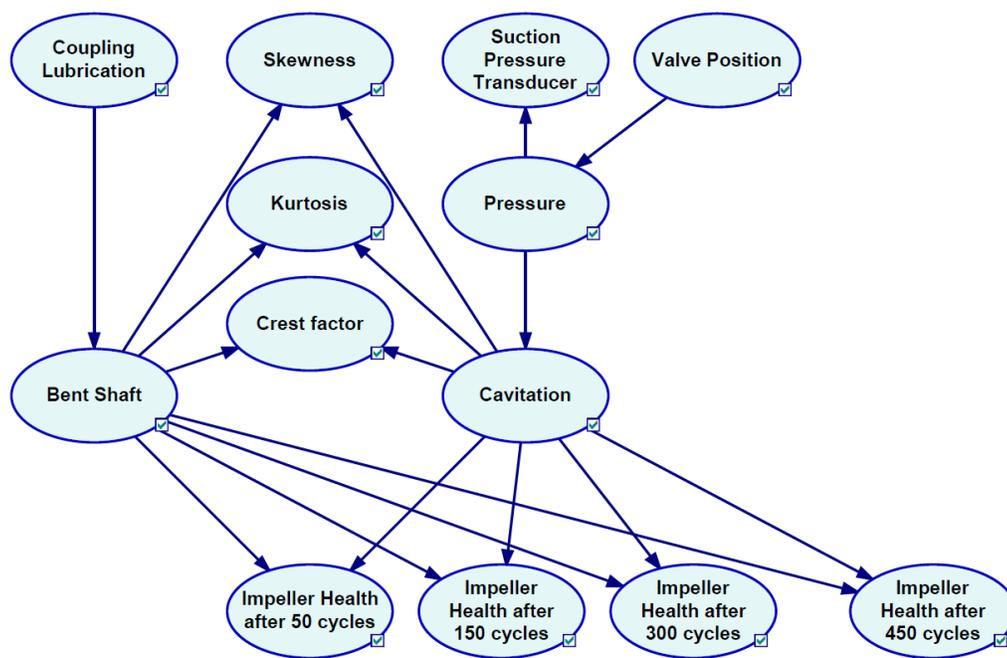
Figure 18: The condition monitoring Bayesian network can diagnose faults, infer root cause of failure, and forecast pump health.
