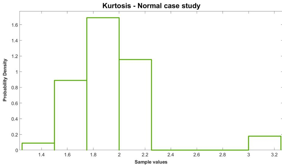
Figure 26: The kurtosis distribution for normal operation is an input for the Bayesian network.
