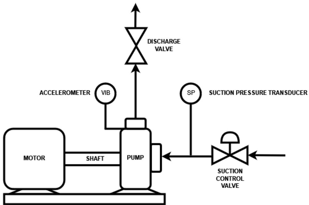
Figure 1: The analyzed pumping system includes a suction valve that controls the flow of water into the pump.
