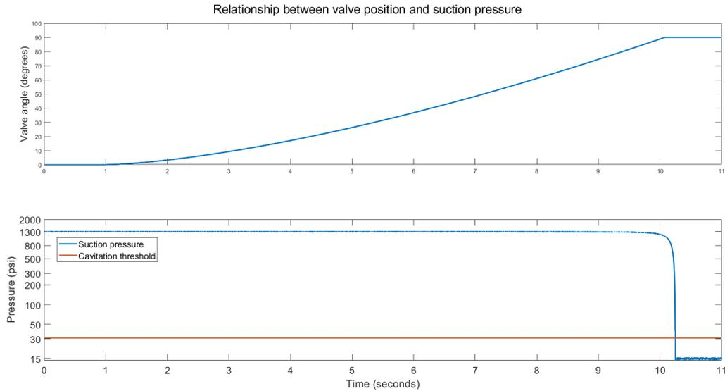
Figure 2: As the suction valve is closed, the pressure through it drops below the liquid vapor pressure.
