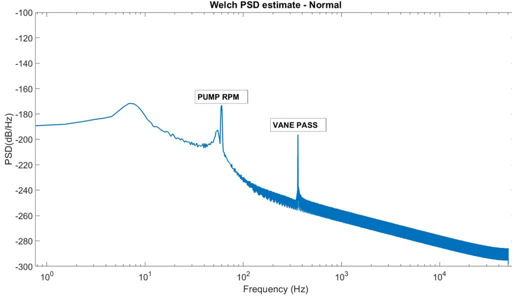
Figure 5: The vibration signal of the pump running during normal operation shows peaks at the vane pass at motor RPM.
