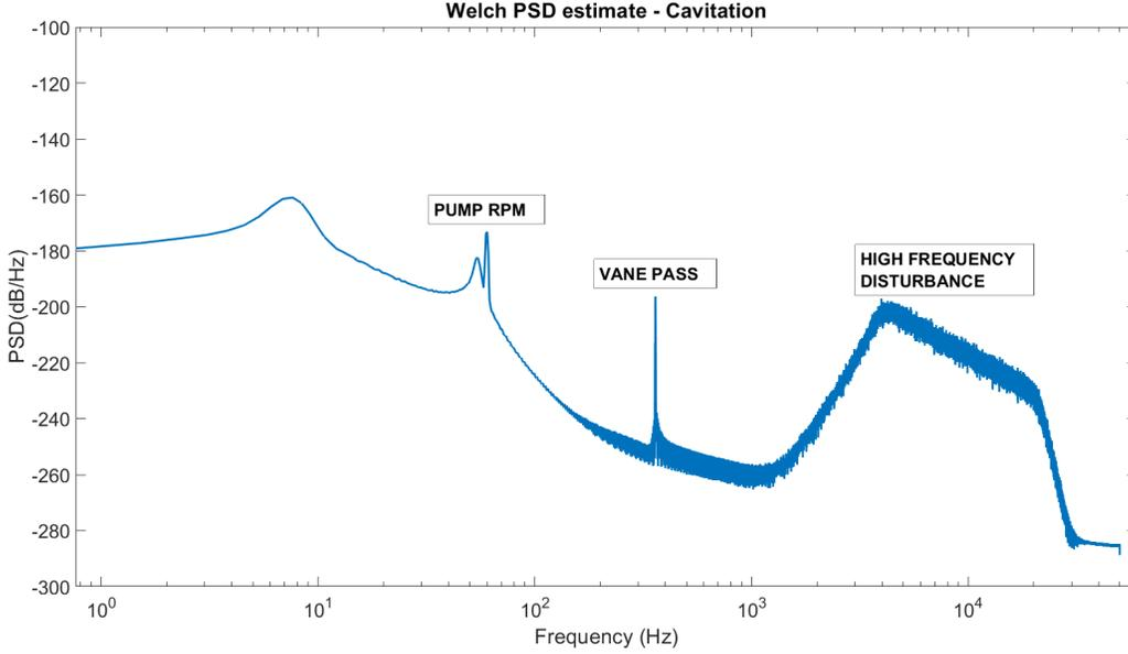
Figure 6: The vibration signal of a cavitating pump shows random high frequency excitation.
