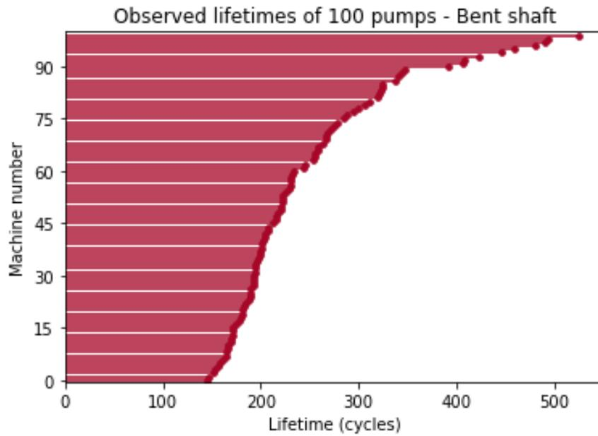
Figure 12: The maximum lifetime of pumps experiencing a bent shaft is around 550 cycles.
