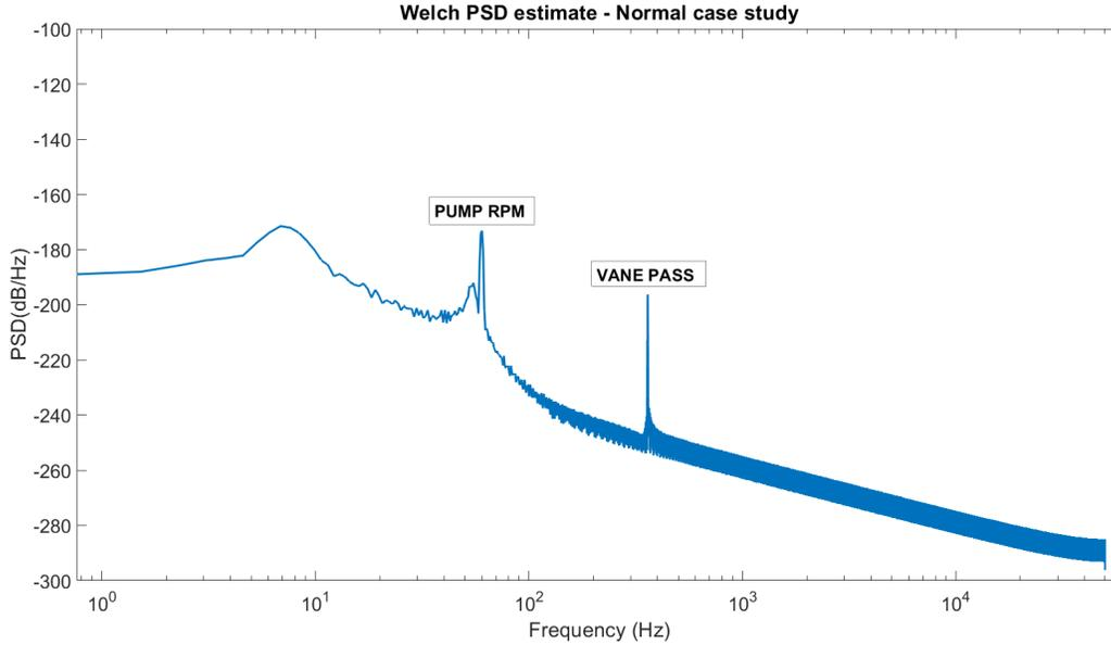
Figure 24: The vane pass and motor RPM frequencies dominate the normal operation vibration response.
