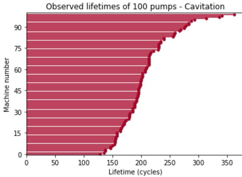
Figure 11: The maximum lifetime of pumps experiencing cavitation is around 400 cycles.
