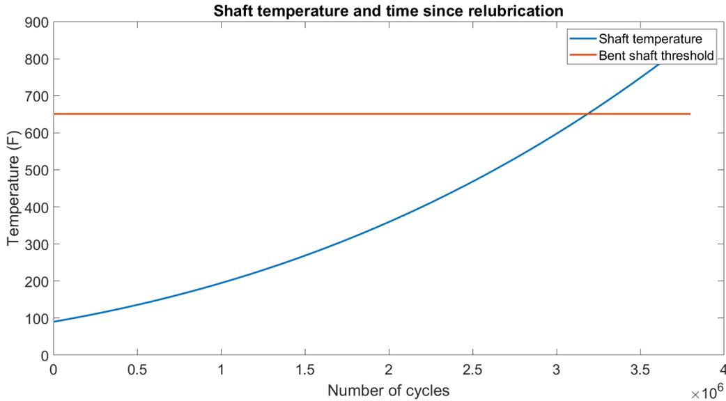
Figure 3: If the pump shaft is not relubricated due to maintenance oversight, it will eventually begin to warp due to thermal expansion.
