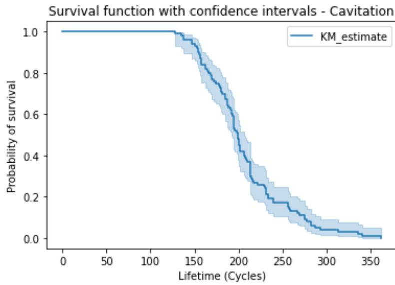
Figure 13: From the Kaplan Meier plot, we determine the median life of cavitating pumps is 200 cycles.
