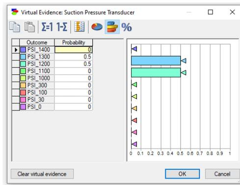
Figure 48: The Suction Pressure Transducer node evidence is set as a distribution.
