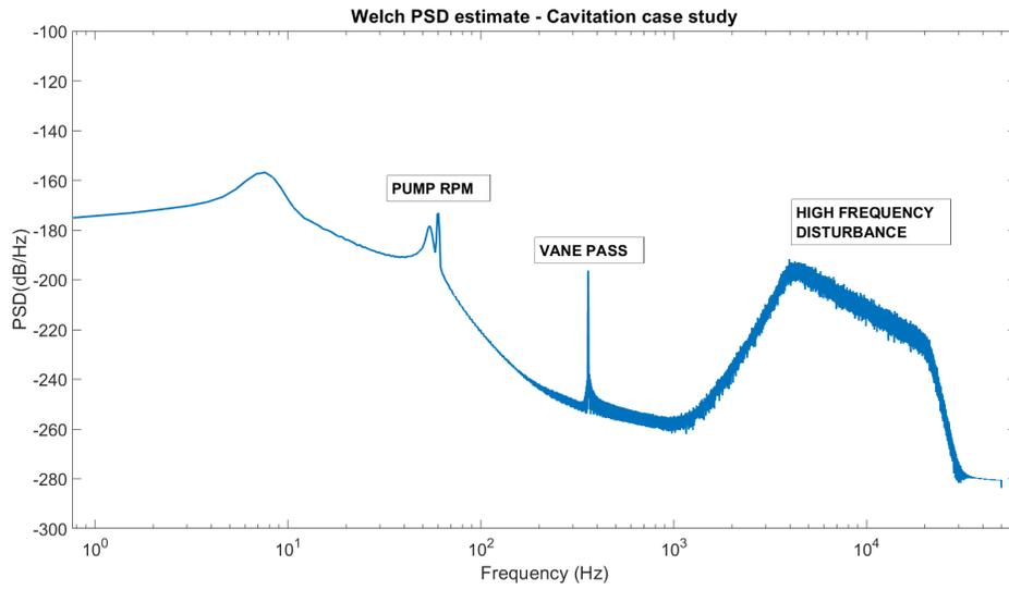
Figure 34: The random high frequencies dominate the cavitation vibration response.
