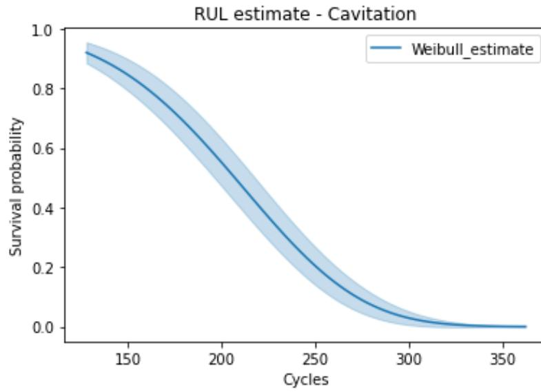
Figure 15: The resulting  $\lambda$  and  $\rho$  values for the cavitation Weibull model are 225.03 and 4.41 respectively.
