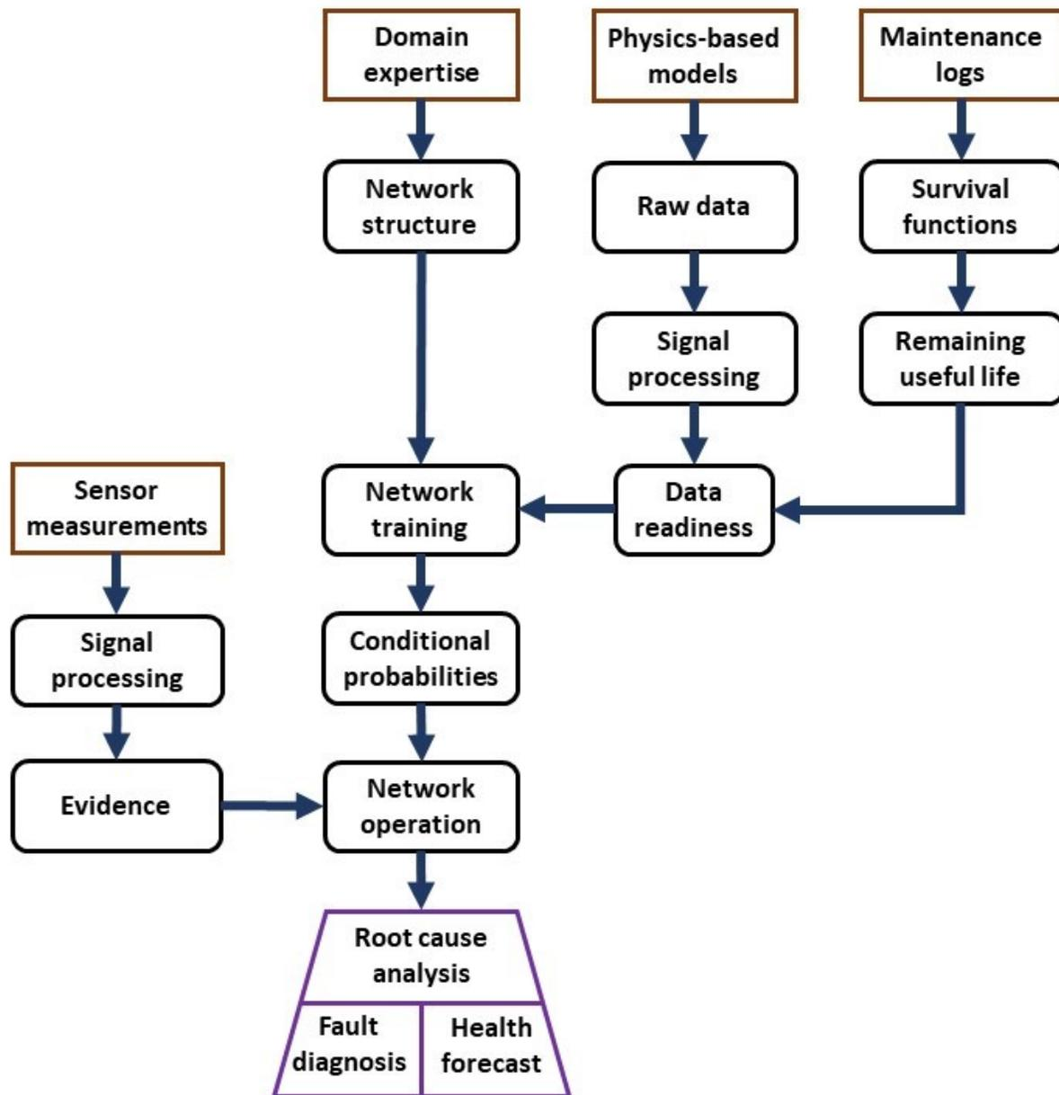
Figure 17: Four disparate systems were combined to develop the final condition monitoring Bayesian network.
