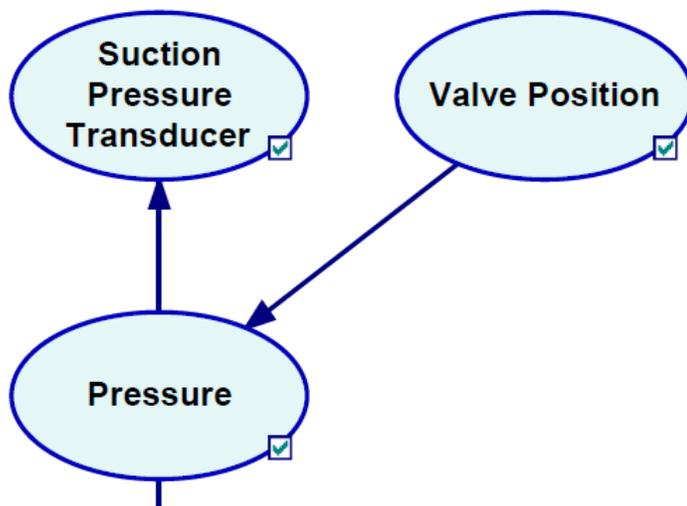
Figure 19: The position of a valve causes a change in the suction pressure.
