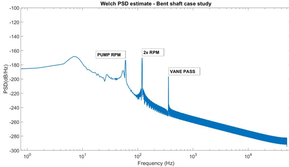
Figure 43: A large amplitude spike at  $2\times$  motor RPM dominates the bent shaft vibration response.
