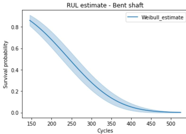
Figure 16: The resulting  $\lambda$  and  $\rho$  values for the bent shaft Weibull model are 276.82 and 2.93 respectively.
