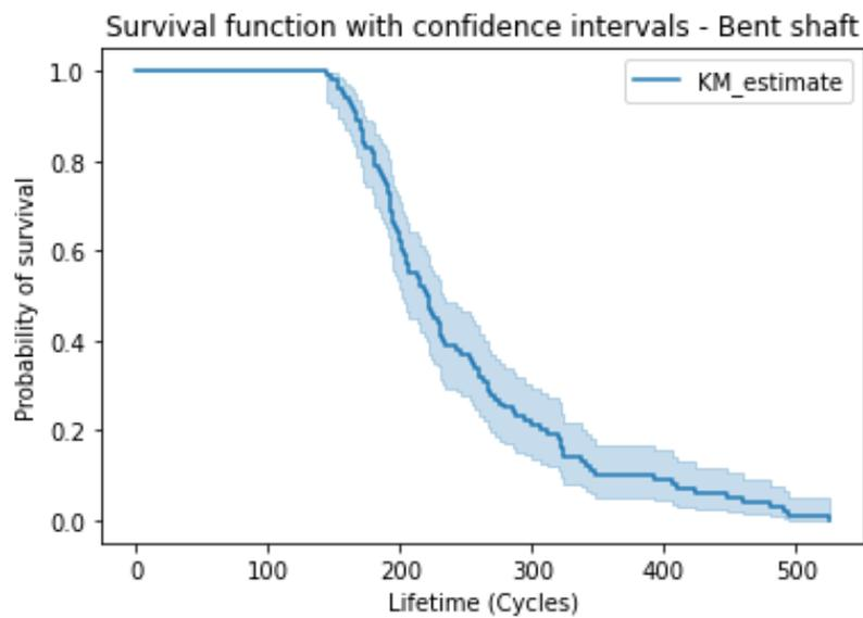
Figure 14: From the Kaplan Meier plot, we determine that half of the pumps fails around 220 cycles while operating with a bent shaft.
