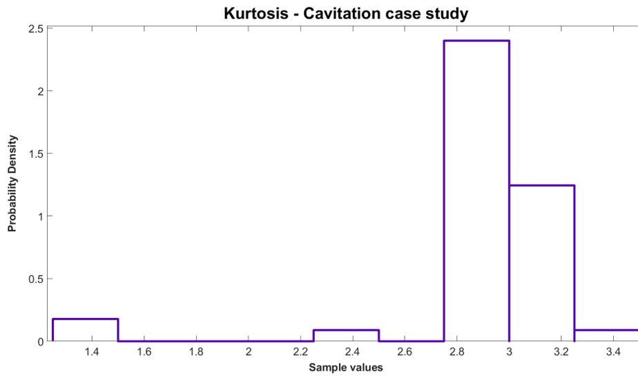
Figure 36: The kurtosis distribution for cavitation is an input for the Bayesian network.
