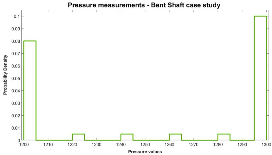
Figure 47: The Suction Pressure Transducer node measurements are input as a distribution.
