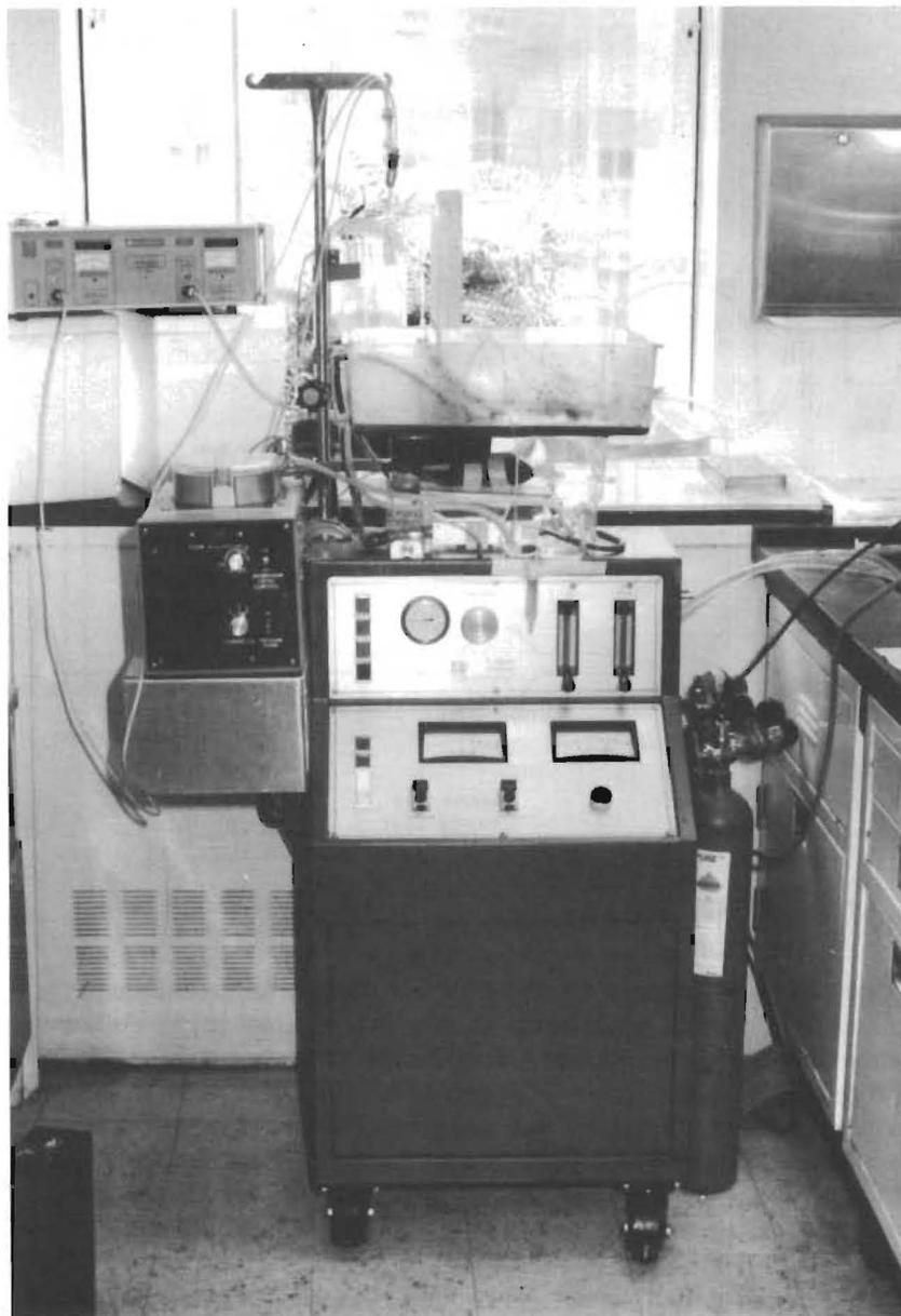
**Figure 1.** Photographic view of the liver perfusion and preservation system developed by modifying a kidney perfusion machine, model MOX-100 (Waters Instruments, Ltd, Rochester, MN).
