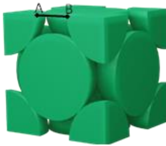
Appendix Figure 1 The face-centered cubic unit cell
