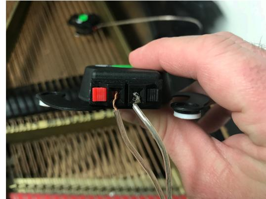
It is also extremely important that the metallic parts of the speaker wires do not touch each other. **DO NOT** do what is pictured below:
