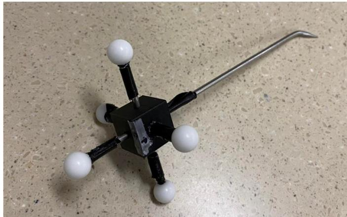
**Figure 13: Custom pointer with array of markers and pointer tip**
