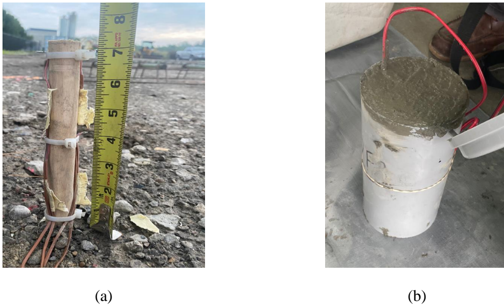
Figure 29: Thermocouple instrumentation in the (a) field and (b) laboratory
