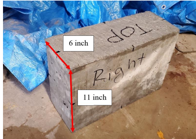
Figure 50: Size effect specimen
