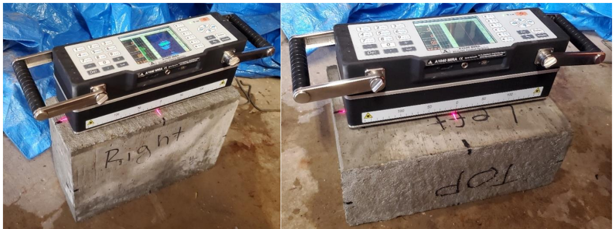
Figure 51: Velocity measurements on a 6-inch side (left) and an 11-inch side (right)
