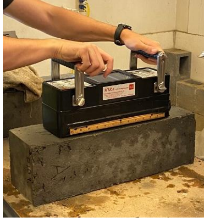
Figure 8: Ultrasonic devices that use shear waves
