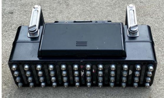
Figure 30: Ultrasonic tomography device, MIRA
