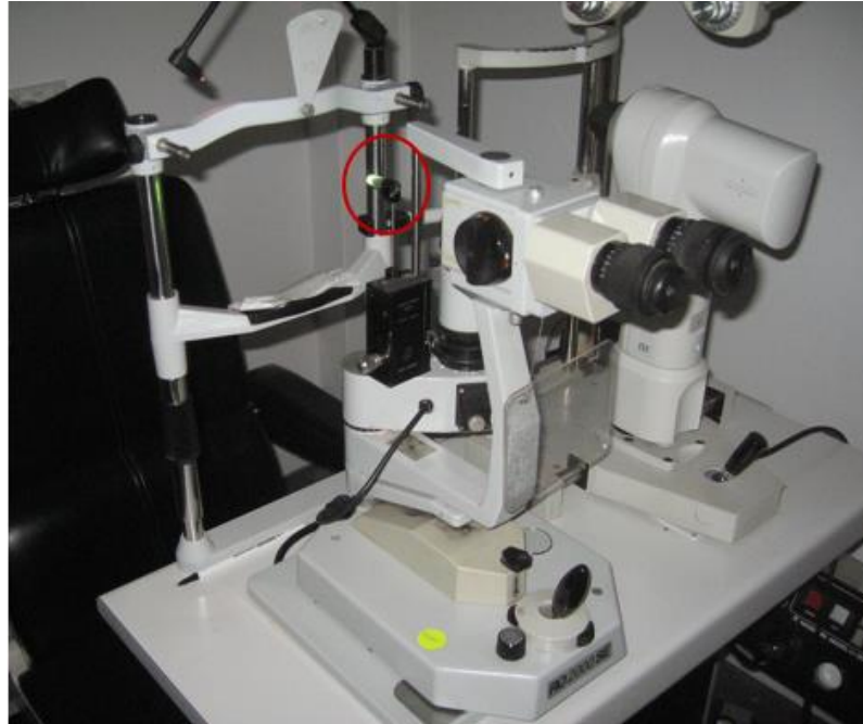
Figure 4 Goldmann applanation tonometer used to measure the internal eye pressure. The component highlighted in the red circle is the tip that would come in contact with the cornea.
