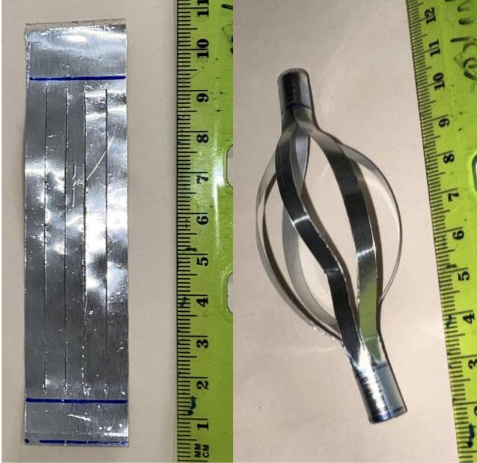
**Figure 32: Lantern-like shape formed from wide bilayer with long slit cutouts.**
