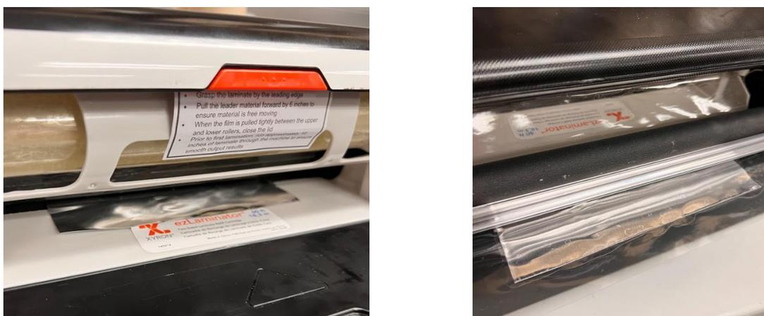
**Figure 7: During lamination. Left: aluminum sheet being fed into back of the laminator. Right: laminated aluminum coming out in front of the laminator.**
