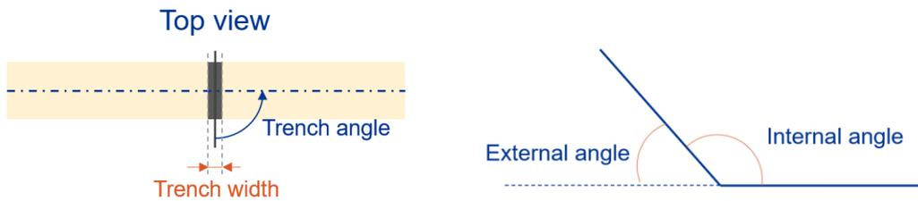
**Figure 25: Properties of trench and definition of bending angles.**
