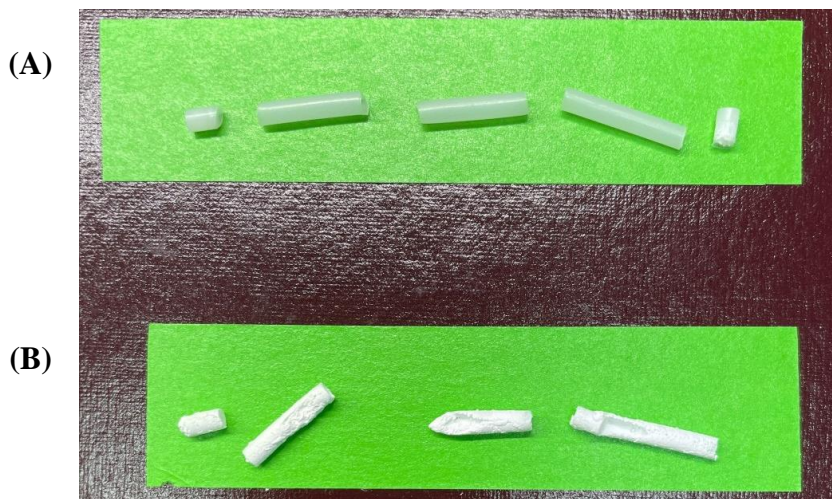
Figure 16 | PCL tubes after extraction by DMSO.
