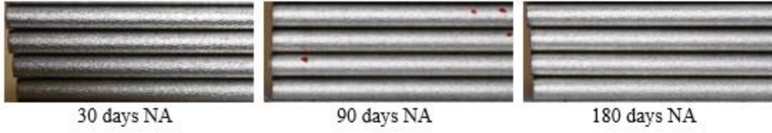
Figure 27: Images of A2_65CW_LF flat hems after 30, 90, and 180 d of natural aging.
