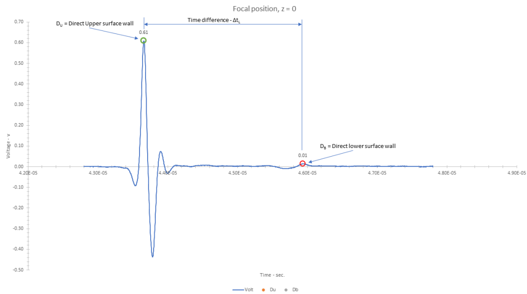
Figure 3-7: Waveform at focal distance for stainless steel SS316L, the defocus
