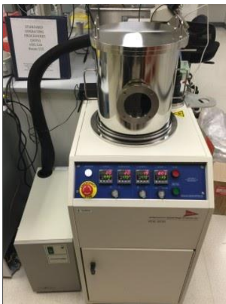
Figure 6-4 PDS 2010 Lab Coater Parylene Deposition System
