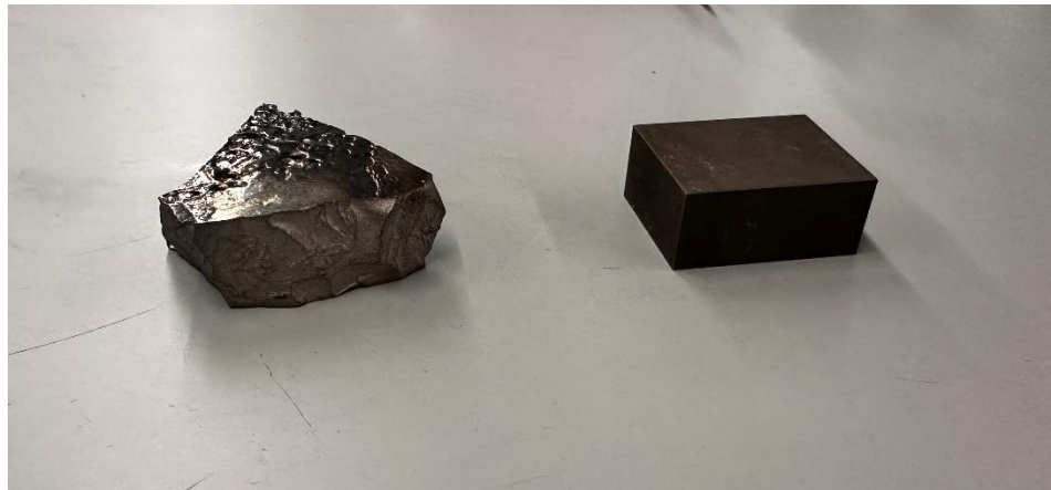
Figure 5-5: Bulk Metallic Glasses Sample 1 - Bulk sample - Ni-based alloy
