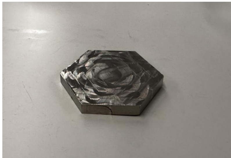
Figure 5-6: Bulk Metallic Glasses Sample 2 - Cracked sample - Zr-based alloy
