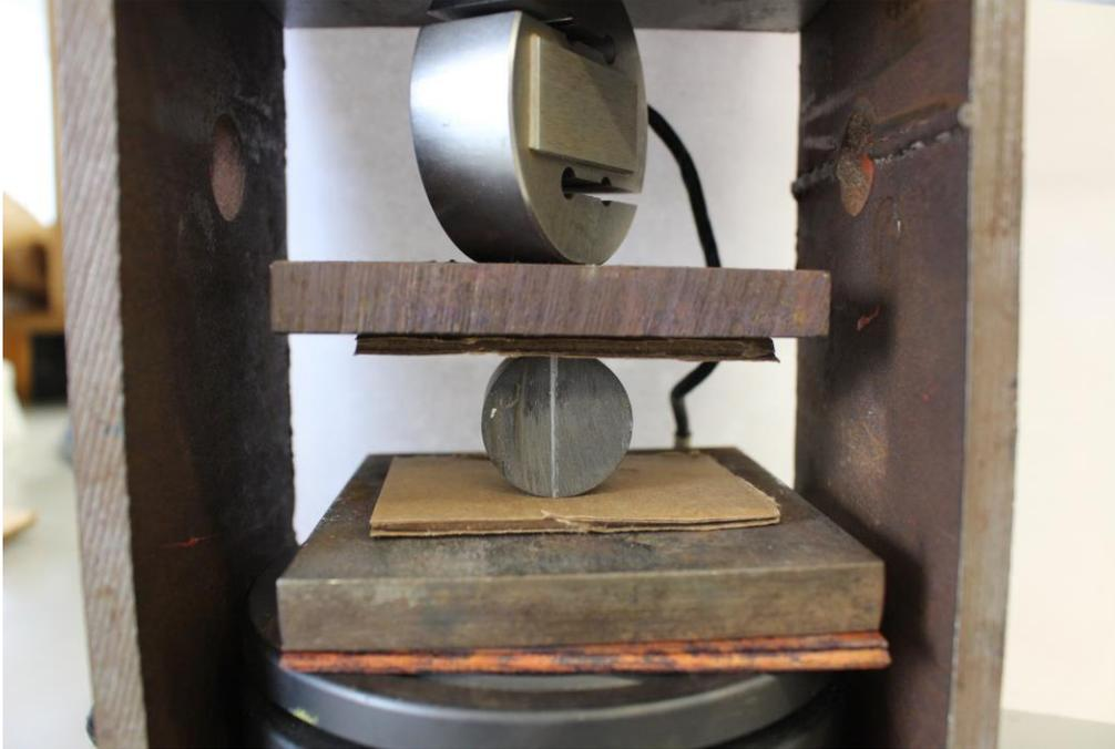
**Figure 2 Tensile sample loaded in frame**
