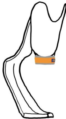
Figure 3 Transtibial IMU Placement
