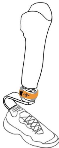
Figure 2 Symes IMU Placement
