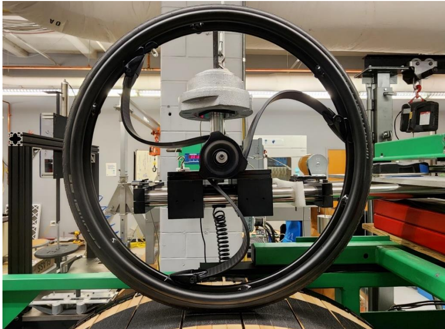
Figure 16: Example set up of the RR drum tester. The configuration shown is with the LoopWheels loaded at 115 lbs.
