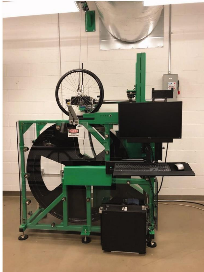
Figure 14: Drum-based rolling resistance tester developed by Ott et al.[61]
