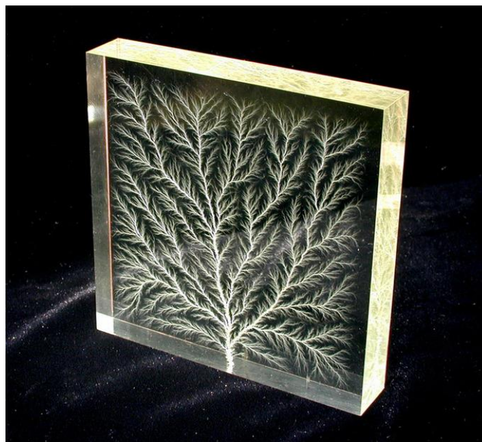
Figure 5: Treelike pattern showing dielectric breakdown in a block of plexiglas, which stems from the root of the breakdown. Figure reproduced from ref. 21
