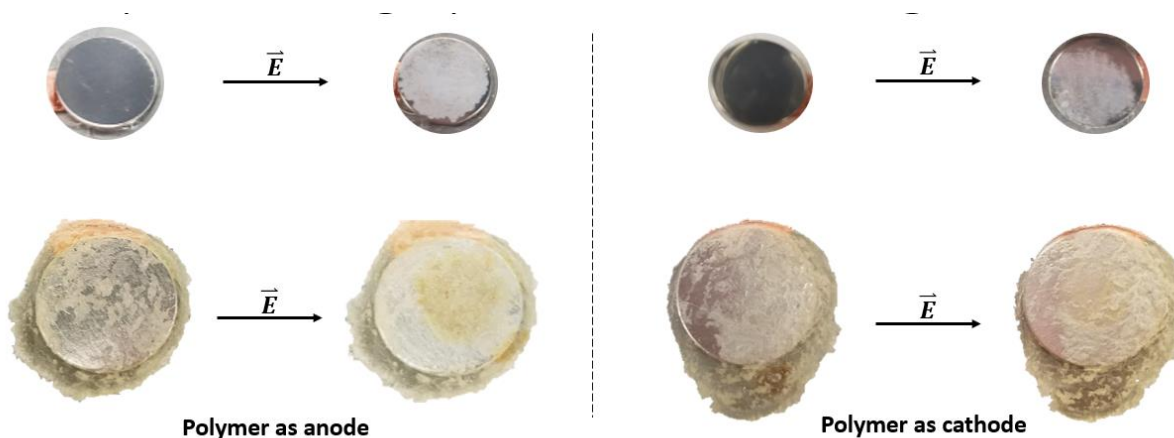
Figure 4.11: When the polymer is the anode, there is significantly more discoloration of the sample bound to the electrode than when the polymer is the anode (the degree of difference somewhat minimized due to lighting issues in these photographs). Both samples show some coating of the unattached electrode.
