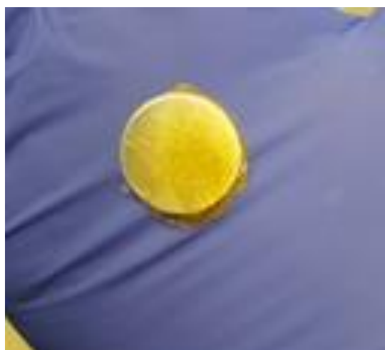
Figure 4.7: Well-bonded film prepared by thermal processing.
