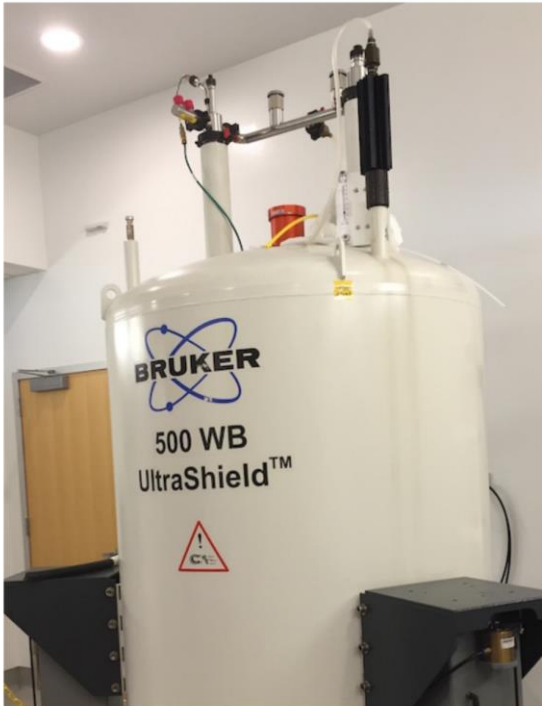
Figure 14 Bruker AV3HD 11.7 tesla/89 mm vertical-bore micro-imaging system
