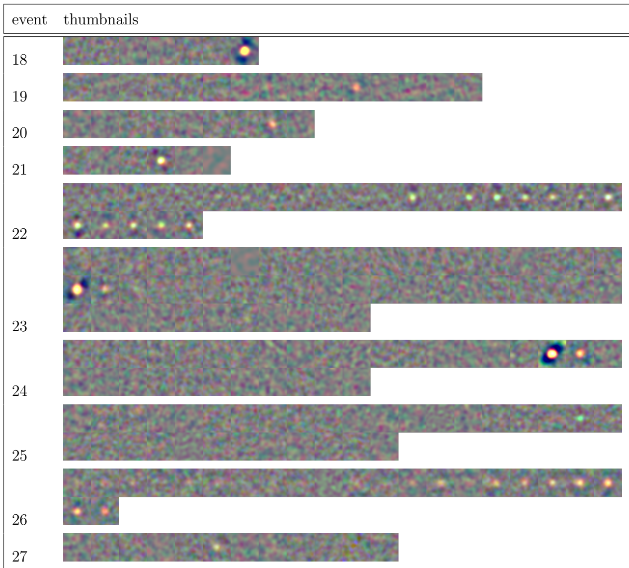
Figure 18: Three color, 10 arcminute by 10 arcminute images of candidates from depth-1 maps about one month before and after detection. Red, blue, and green correspond to f090, f150, and f220 respectively. Note the thumbnails are chronological but have inconsistent spacing in time. These plots are included for illustration rather than quantitative analysis.
