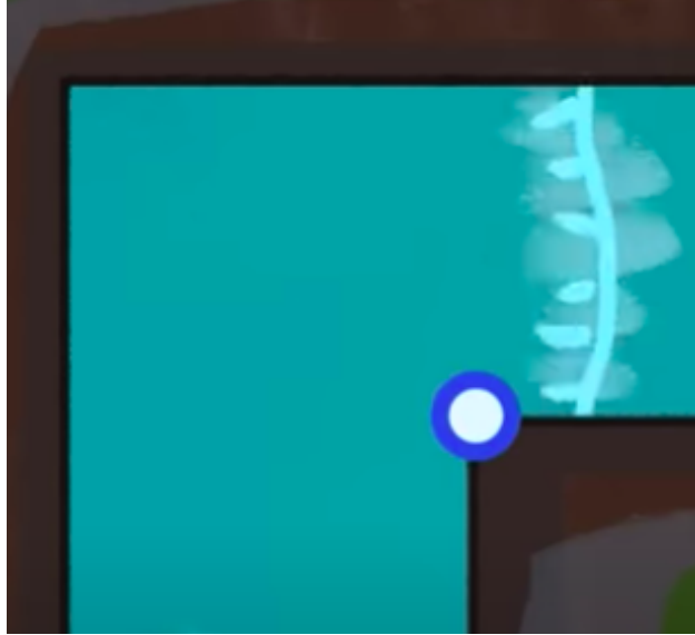
Figure 1: Without the appropriate boundary condition (in addition to the obligatory slip condition), the Navier-Stokes equations will predict that the velocity field diverges to infinity in the indicated inside corner.
