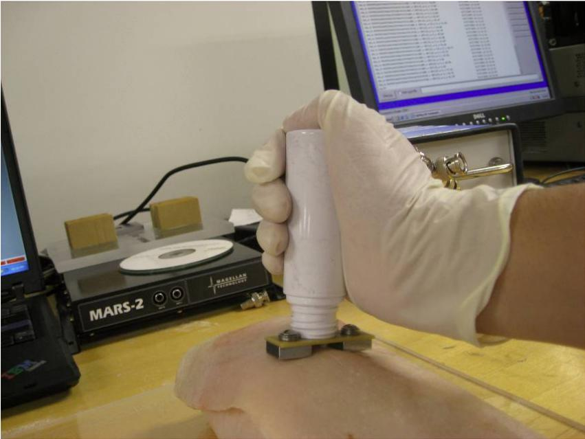
**Figure 37.** Experiment on a UHF system: knee implant wrapped by pig skin
