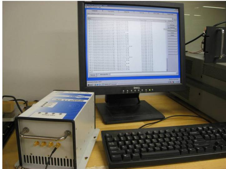
**Figure 3.** The SAMSys UHF RFID system
