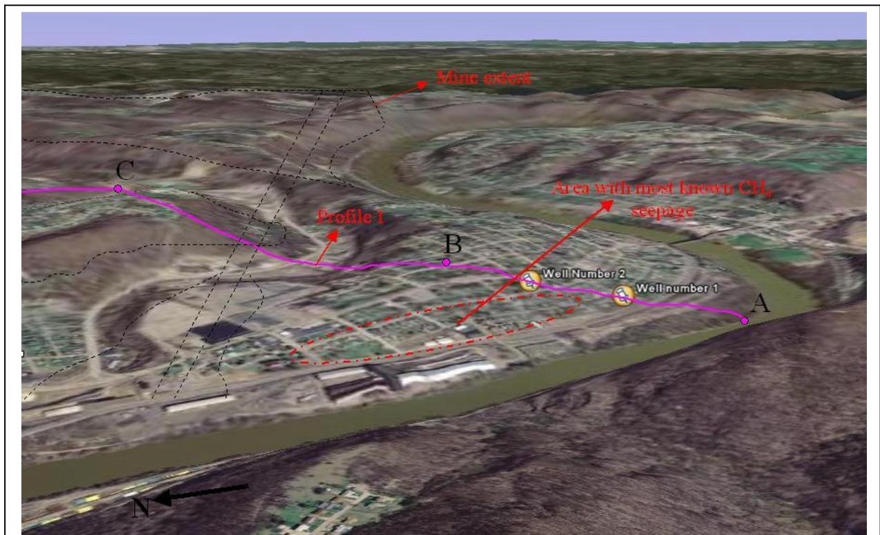
**Figure 72.** Profile across Versailles, PA: (A): Youghiogheny River level; (B): Top of the first hill; (C): Top of the second hill. Dashed line schematically pictures the extent of existing mine.
