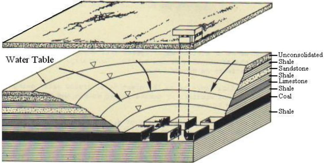
**Figure 74.** Drawdown of groundwater table due to underground mining operations (Stephenson et al, 1981).
