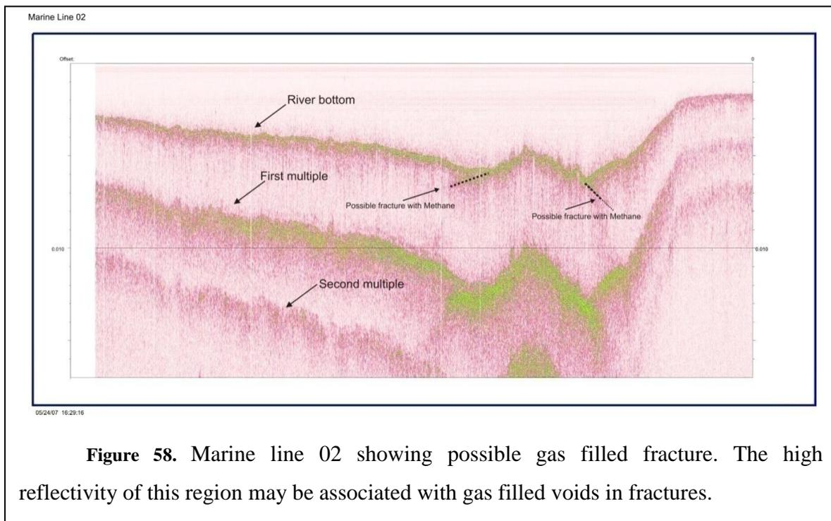
**Figure 58.** Marine line 02 showing possible gas filled fracture. The high reflectivity of this region may be associated with gas filled voids in fractures.
