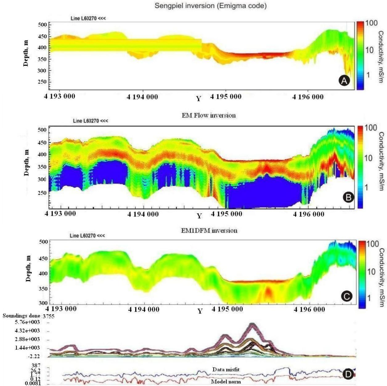
**Figure 17.** Conductivity depth images derived from three different inversion algorithms applied to flight line 60270. (A): Sengpiel technique. (B): EM Flow algorithm. (C): EM1DFM inversion with stabilization functional. (D): Data misfit and model norm for EM1DFM inversion are plotted for each observation point.
