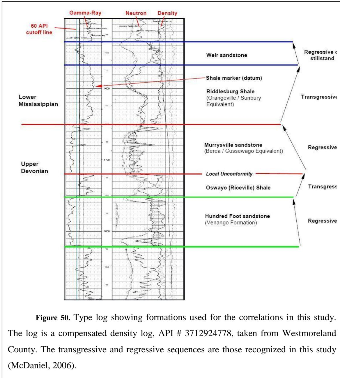
**Figure 50.** Type log showing formations used for the correlations in this study. The log is a compensated density log, API # 3712924778, taken from Westmoreland County. The transgressive and regressive sequences are those recognized in this study (McDaniel, 2006).
