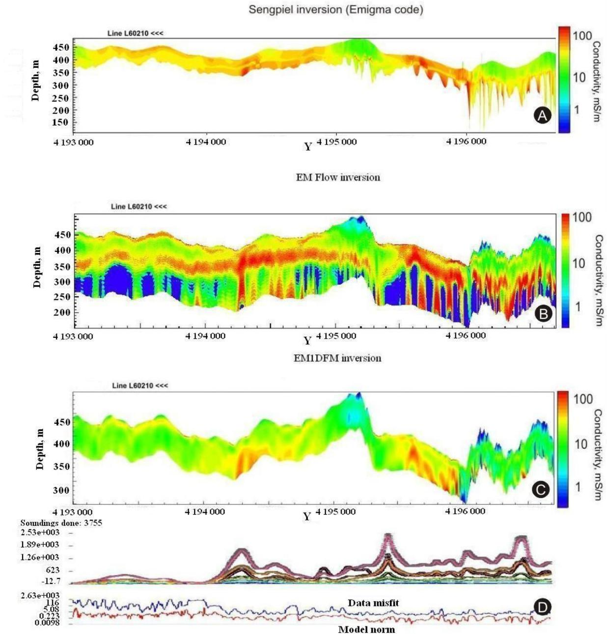
**Figure 16.** Conductivity depth images derived from three different inversion algorithms applied to flight line 60210. (A): Sengpiel technique. (B): EM Flow algorithm. (C): EM1DFM inversion with stabilization functional. (D): Data misfit and model norm for EM1DFM inversion are plotted for each observation point.
