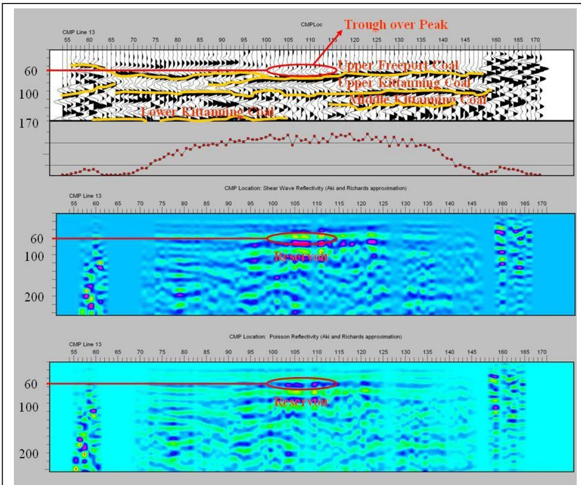
**Figure 68.** Shear wave reflectivity and Poisson reflectivity from CMP line 13 of the 3D reflection seismic survey. Enhanced parameter variation is observed between CMP locations 100 to 115.
