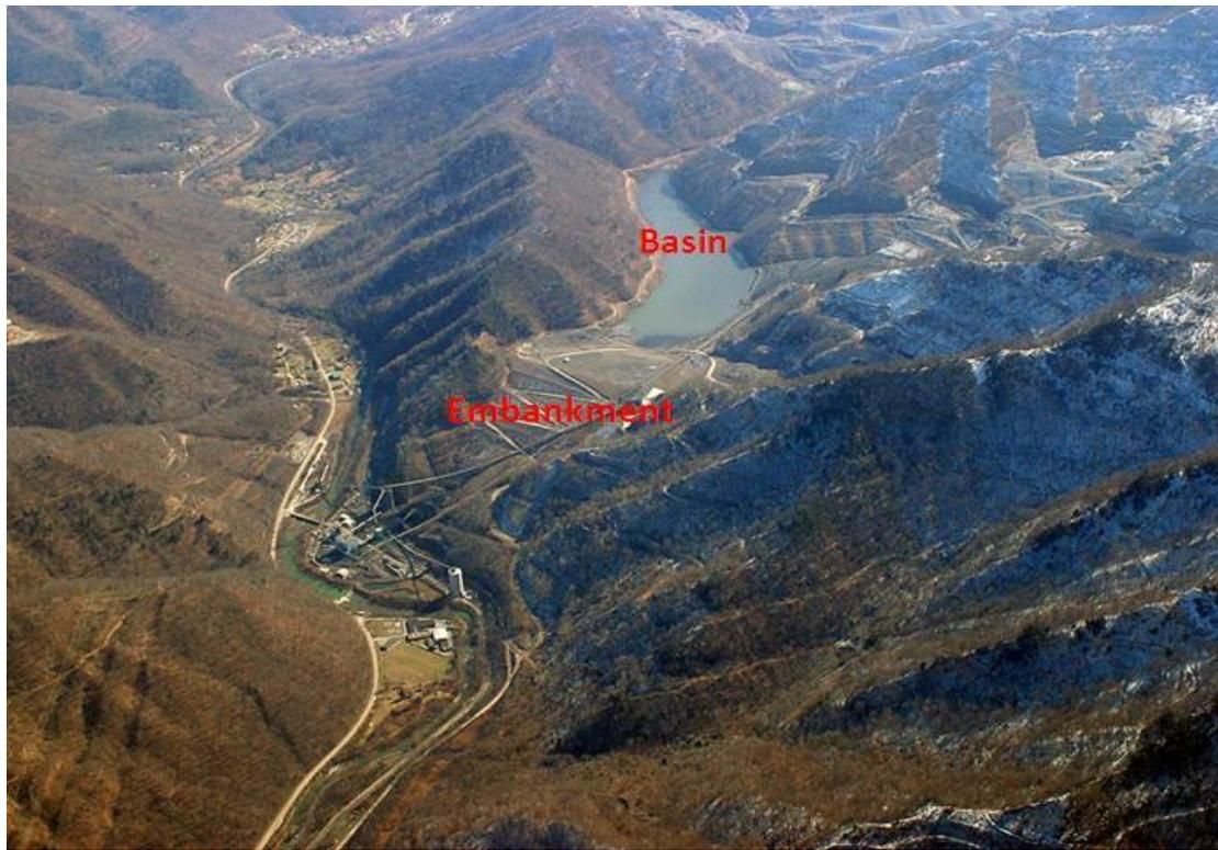
**Figure 2.** An aerial photograph of an upstream raised coal waste impoundment; two main components are outlined here: basin and embankment.
