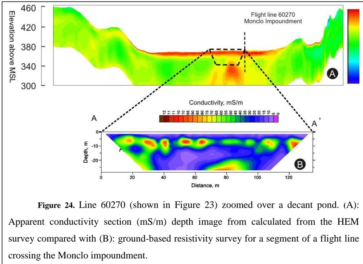
**Figure 24.** Line 60270 (shown in Figure 23) zoomed over a decant pond. (A): Apparent conductivity section (mS/m) depth image from calculated from the HEM survey compared with (B): ground-based resistivity survey for a segment of a flight line crossing the Monclo impoundment.
