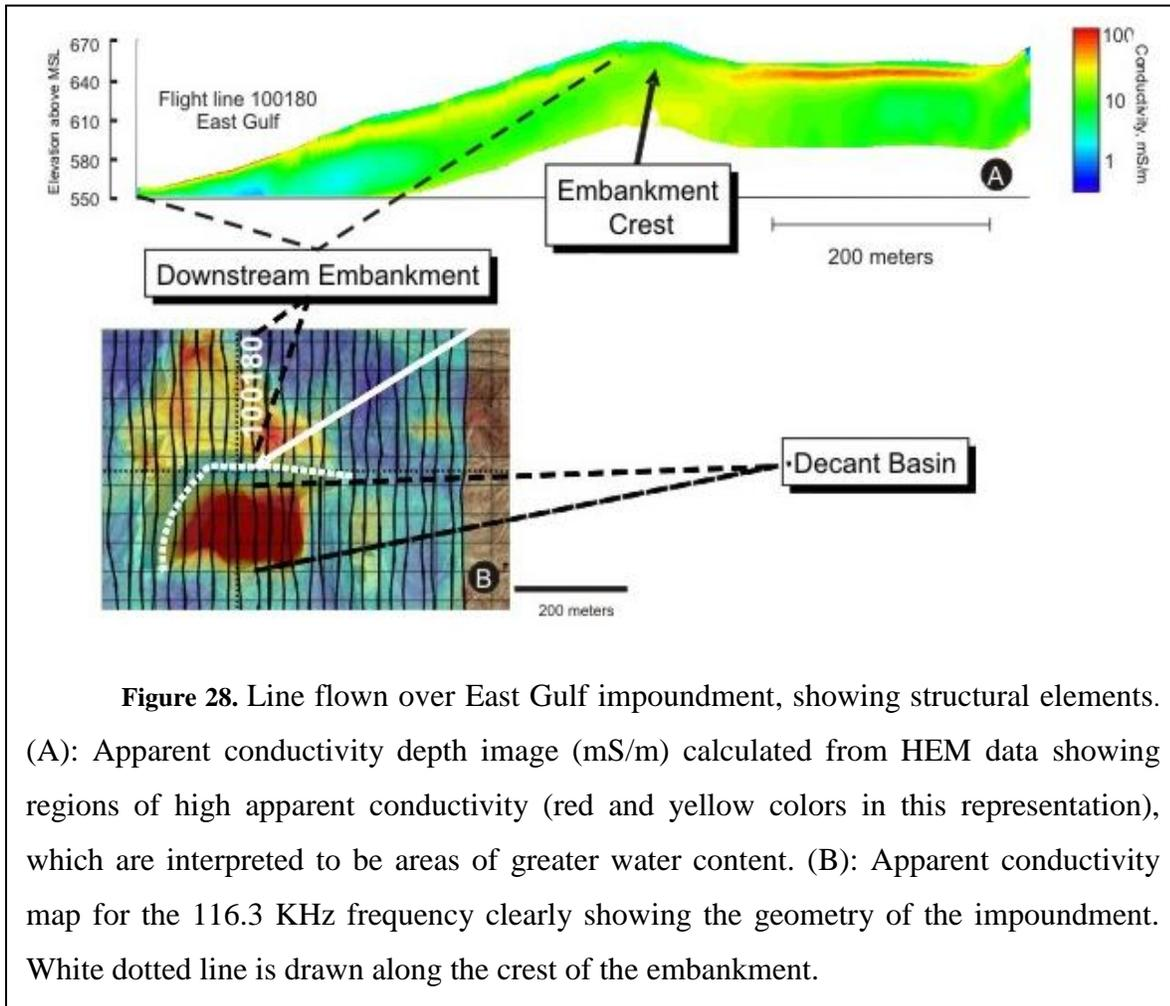
**Figure 28.** Line flown over East Gulf impoundment, showing structural elements. (A): Apparent conductivity depth image (mS/m) calculated from HEM data showing regions of high apparent conductivity (red and yellow colors in this representation), which are interpreted to be areas of greater water content. (B): Apparent conductivity map for the 116.3 KHz frequency clearly showing the geometry of the impoundment. White dotted line is drawn along the crest of the embankment.
