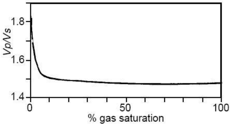
**Figure 42.** Dependence of  $V_p/V_s$  ratio with respect to the percentage of gas content in groundwater saturated sandstone (Ostrander, 1984).
