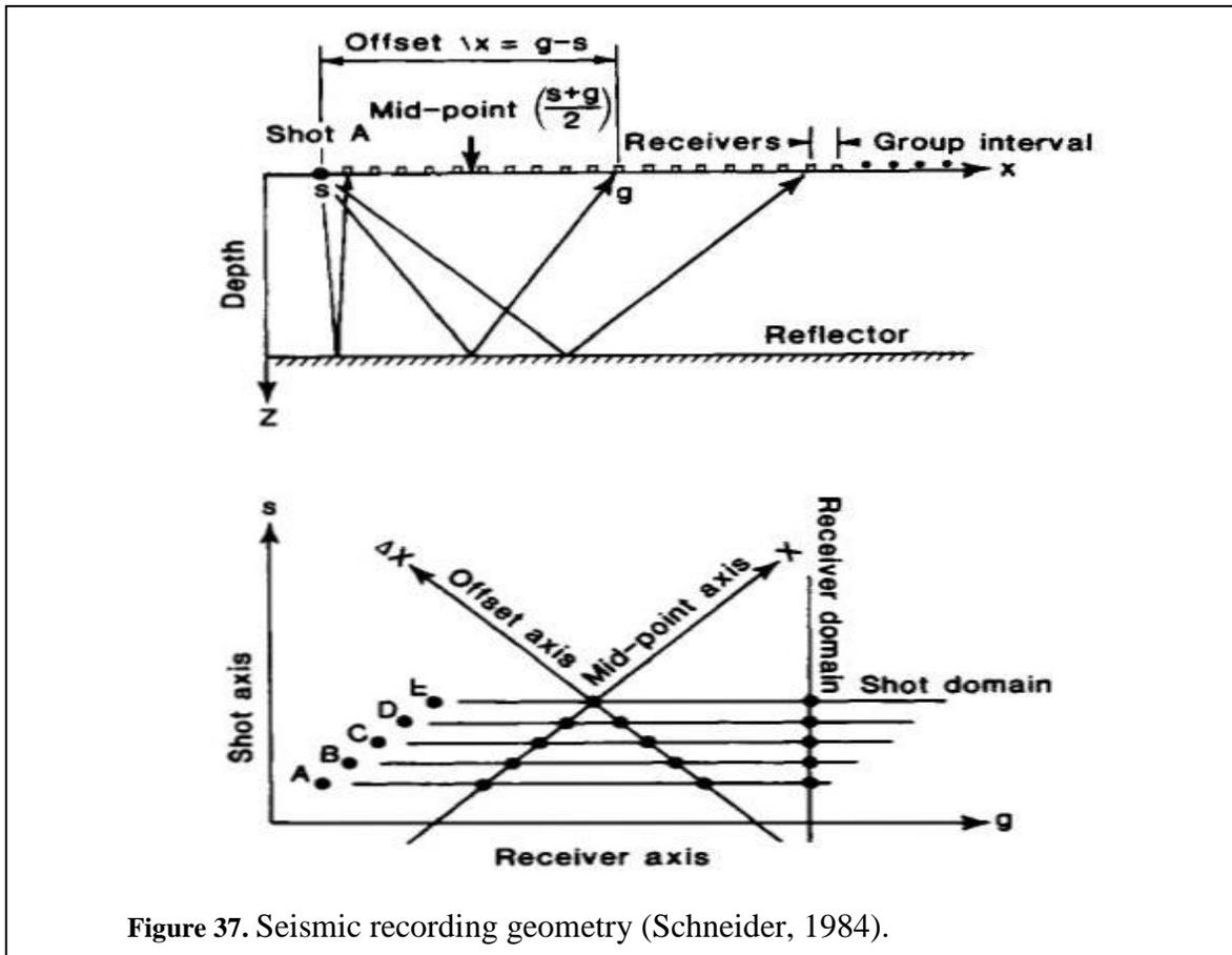
Figure 37. Seismic recording geometry (Schneider, 1984).
