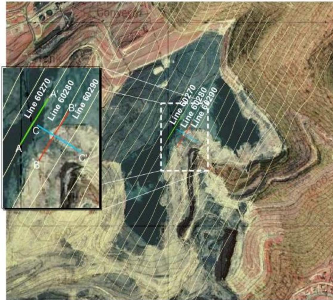
**Figure 23.** Digital orthophoto of the Monclo impoundment near Sharples, WV showing the locations of flight lines from the helicopter survey (light yellow). Inset map shows the location of three resistivity profiles (AA',BB' and CC') that were acquired using DC resistivity method to corroborate helicopter survey results.
