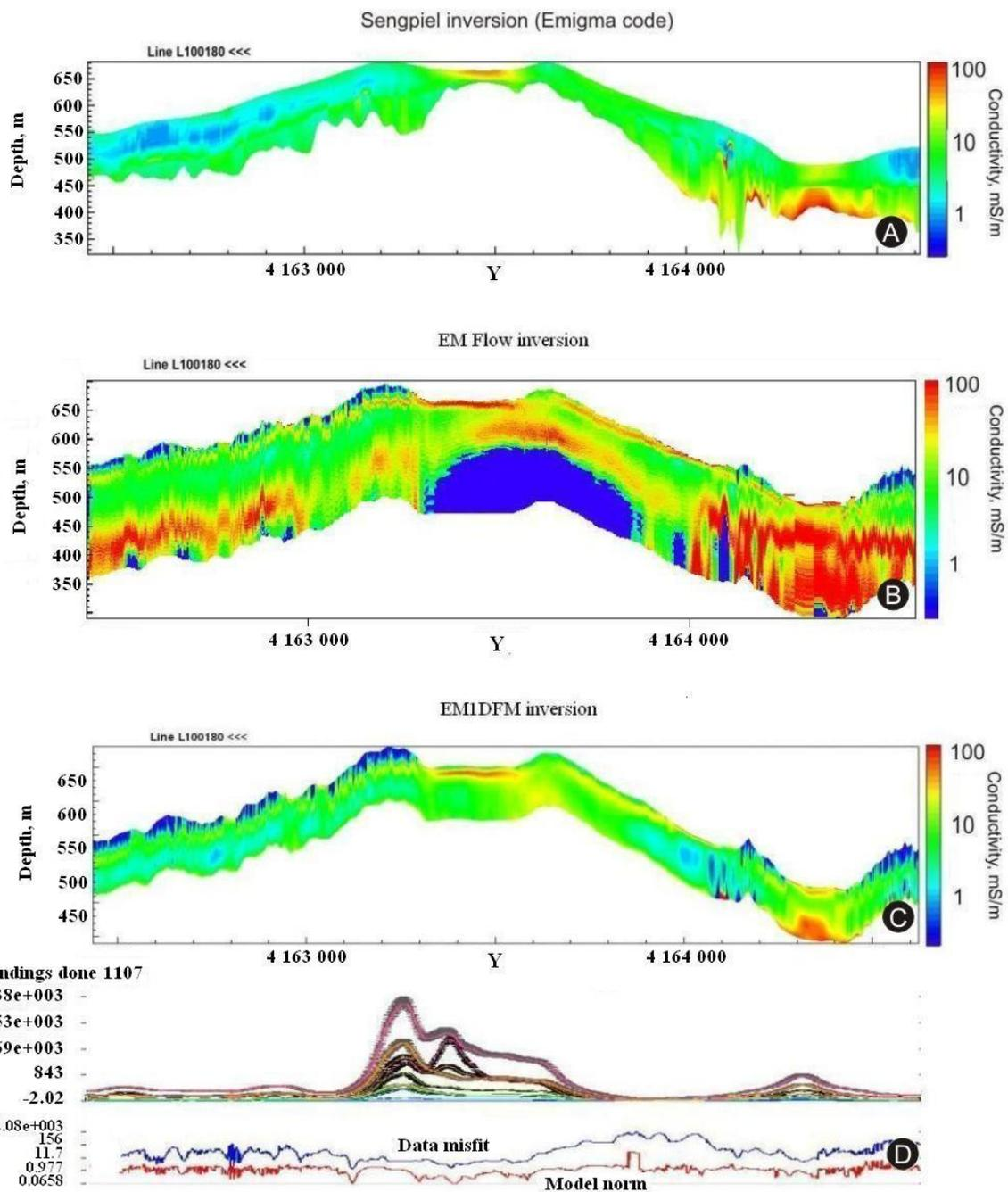
**Figure 20.** Conductivity depth images derived from three different inversion algorithms applied to flight line 100180. (A): Sengpiel technique. (B): EM Flow algorithm. (C): EM1DFM inversion with stabilization functional. (D): Data misfit and model norm for EM1DFM inversion are plotted for each observation point.
