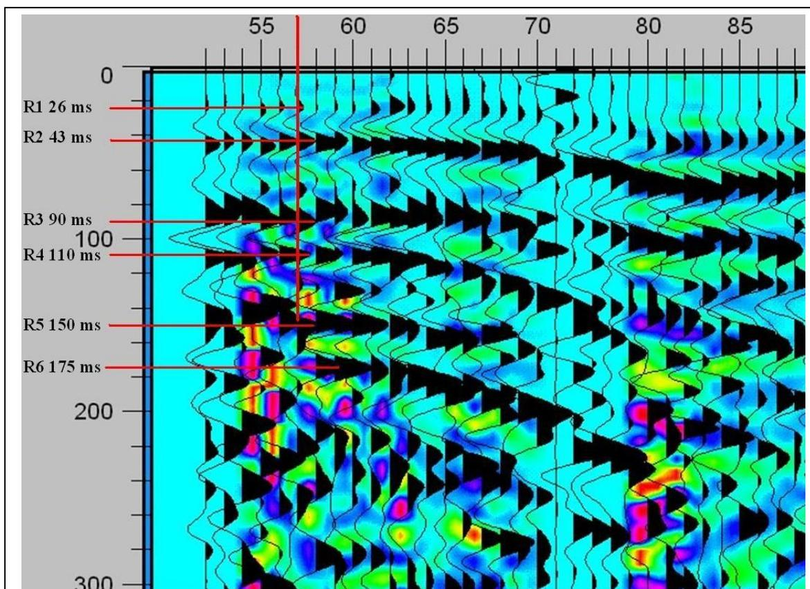
**Figure 66.** Delineation of six reflectors from the reflection seismic record derived from CMP line 9. Shaded peaks represent maximums of reflection coefficient, which according to our calculations should correspond to coal beds, exceeding 3.45 m in thickness.
