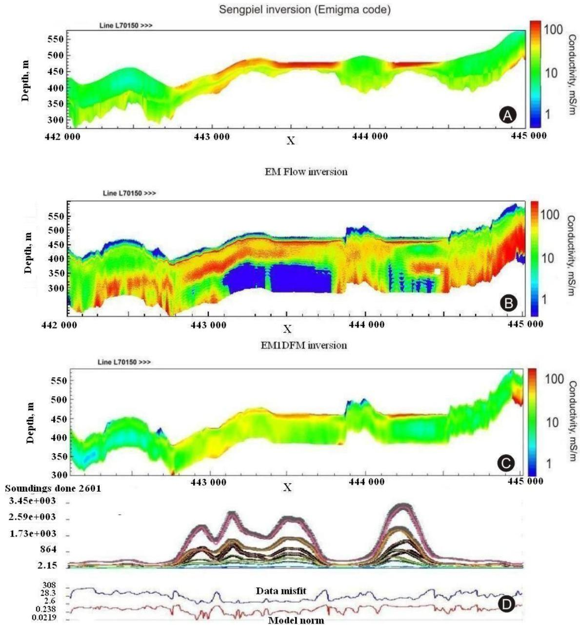
**Figure 19.** Conductivity depth images derived from three different inversion algorithms applied to flight line 70150. (A): Sengpiel technique. (B): EM Flow algorithm. (C): EM1DFM inversion with stabilization functional. (D): Data misfit and model norm for EM1DFM inversion are plotted for each observation point.
