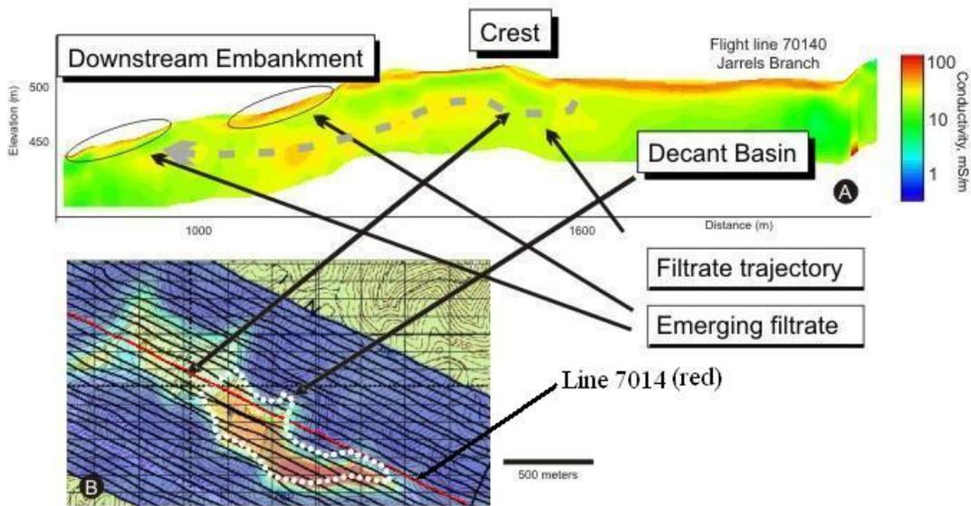
**Figure 30.** (A): Apparent conductivity depth image (mS/m) calculated from HEM data collected over Jarrell's Branch impoundment showing regions of high apparent conductivity (red and yellow colors in this representation). Filtrate flow trajectory is delineated on the image as well as areas of emerging filtrate. (B): Apparent conductivity map for the highest frequency collected clearly showing the geometry of the impoundment.
