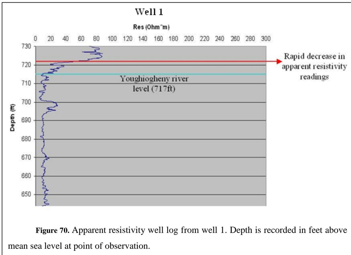
**Figure 70.** Apparent resistivity well log from well 1. Depth is recorded in feet above mean sea level at point of observation.
