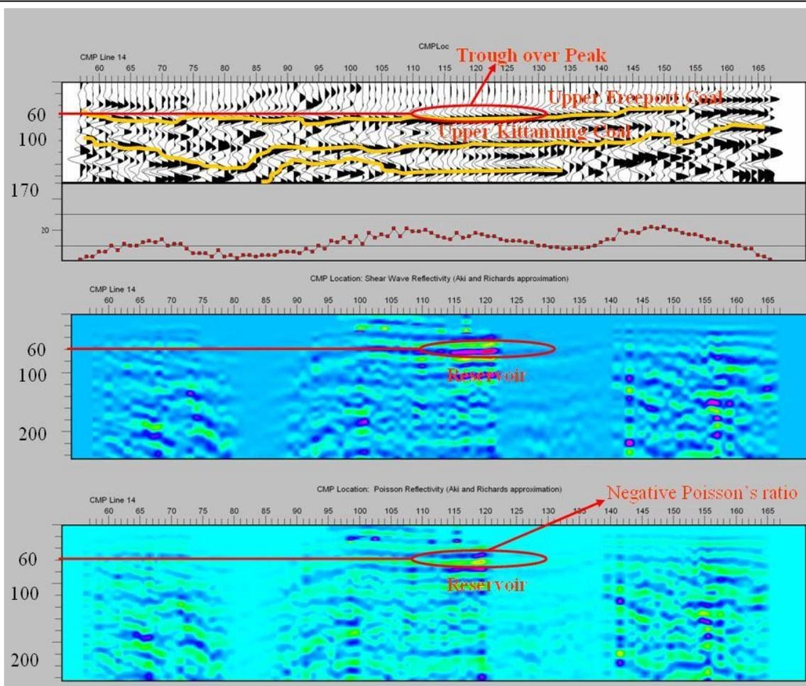
**Figure 69.** Seismic interpretation of line 14 (shallow reservoir). Enhanced parameter variation is observed between CMP locations 110 to 130.
