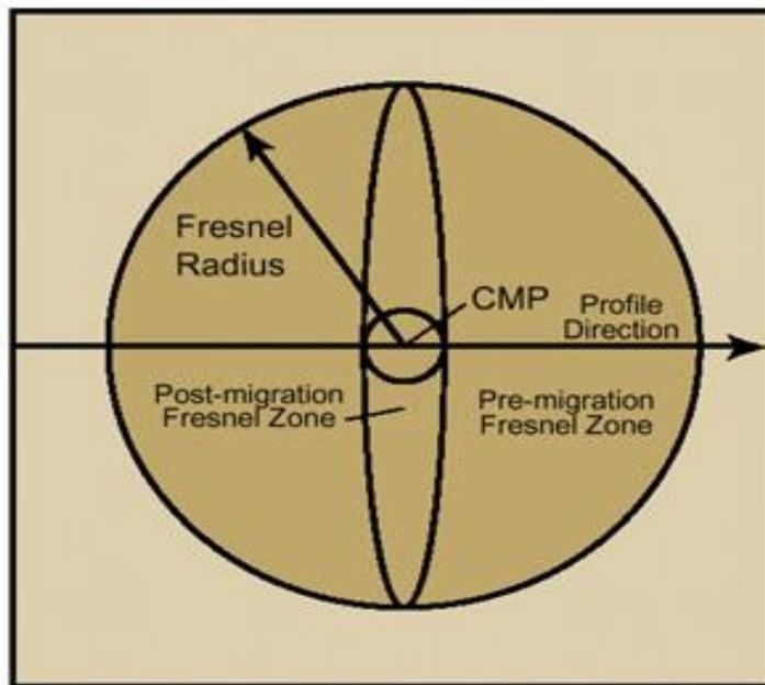
**Figure 39.** Decreasing radius of Fresnel zone (increasing horizontal resolution) by implementing 2D and 3D migration. 2D migration allows to decrease Fresnel zone in 1 direction (to an ellipse), while 3D migration allows to narrow the zone down to a smaller circle (Sheriff, 1991).
