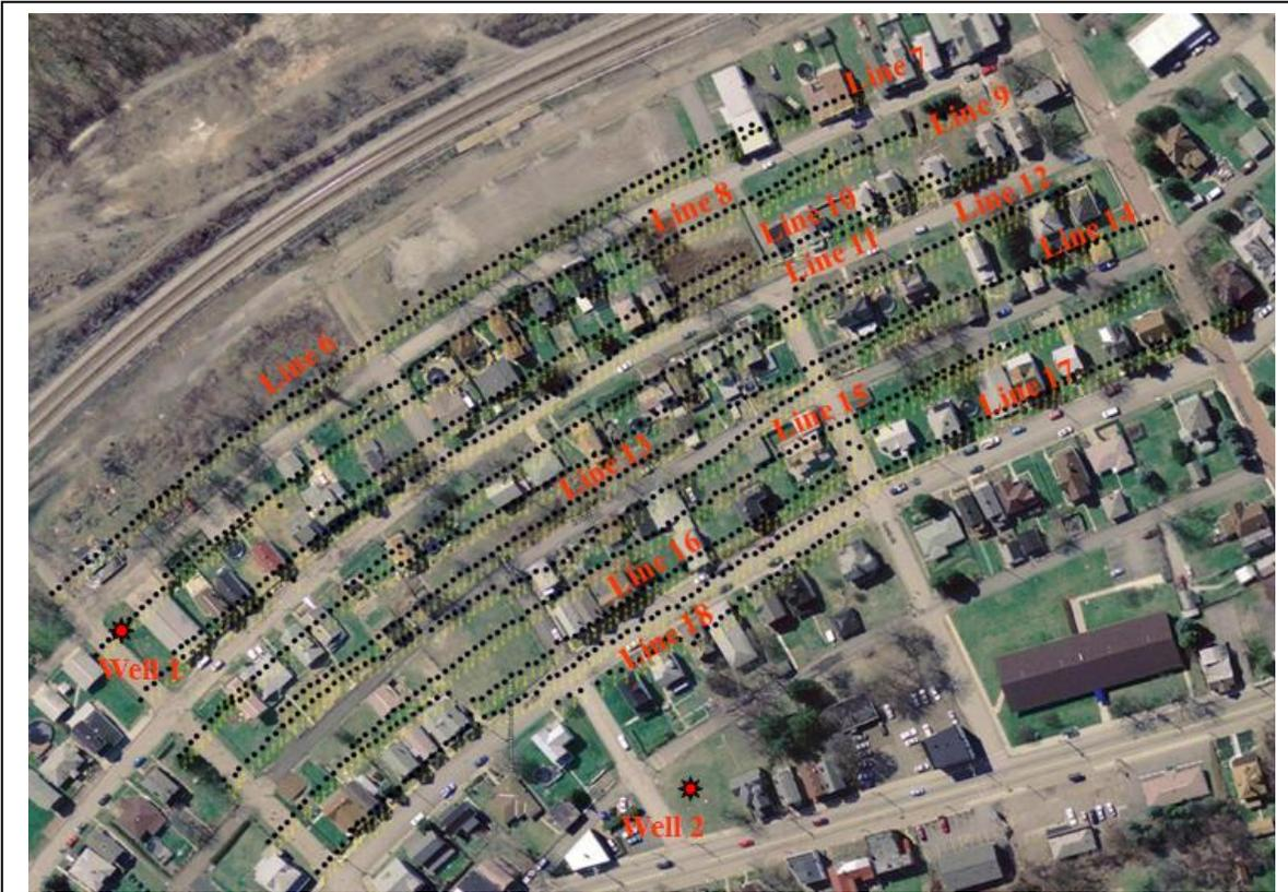
**Figure 61.** Common midpoint locations. Four energy lines and three geophone lines resulted in a total of 12 CMP lines, approximately 25 m apart from one another.
