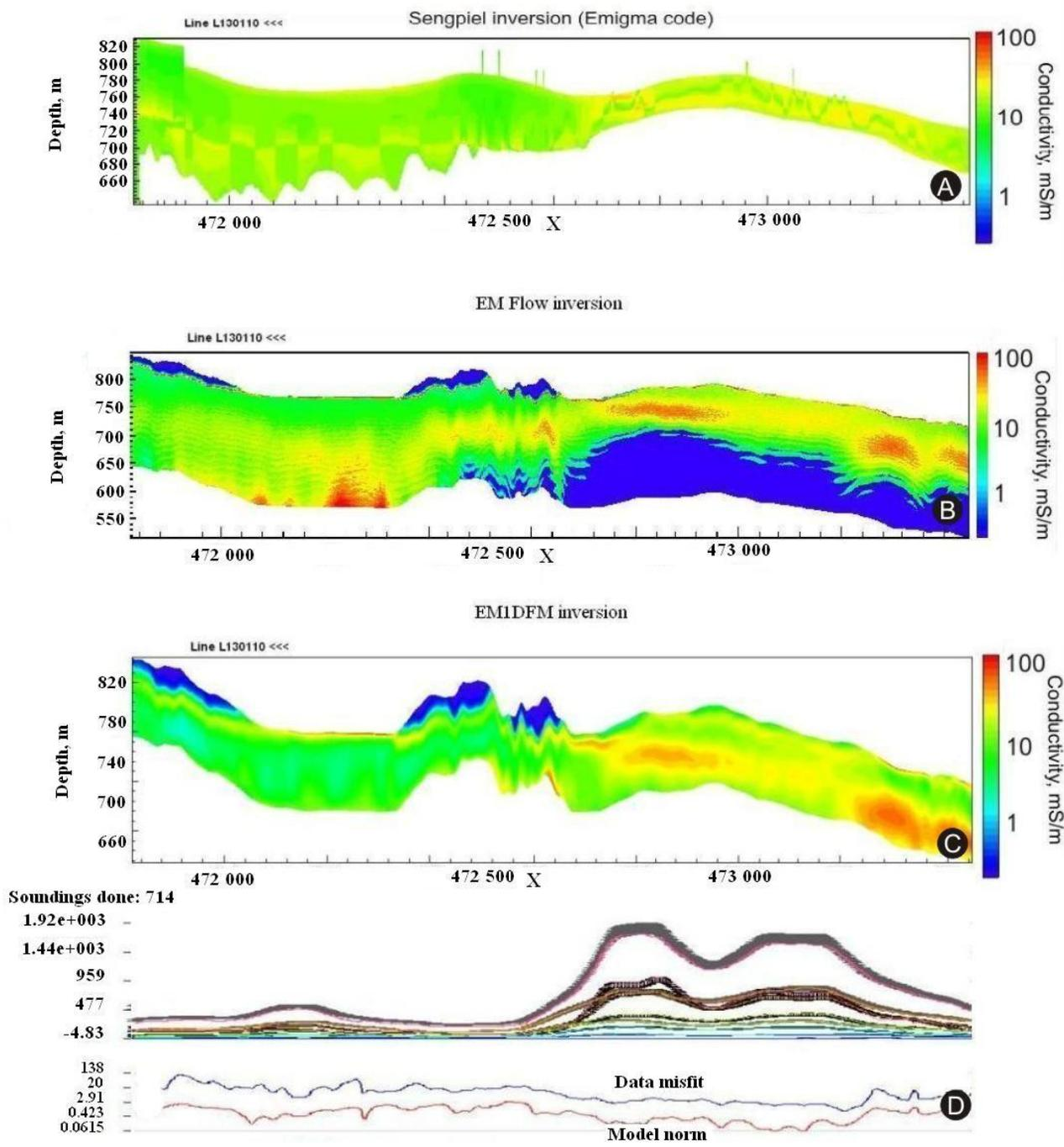
**Figure 21.** Conductivity depth images derived from three different inversion algorithms applied to flight line 130110. (A): Sengpiel technique. (B): EM Flow algorithm. (C): EM1DFM inversion with stabilization functional. (D): Data misfit and model norm for EM1DFM inversion are plotted for each observation point.
