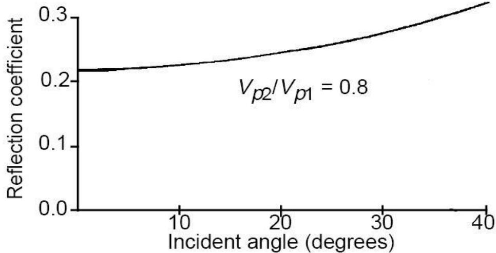
**Figure 41.** Dependence of the absolute value of the reflection coefficient from the angle of incidence. This relationship was shown by Ostrander (1984) for a specific case ( $V_{p2}/V_{p1} = 0.8$ ), where  $V_{p2}$  is the velocity of P-wave in a sandstone and  $V_{p1}$  – is velocity of P-wave in a sealing shale unit.
