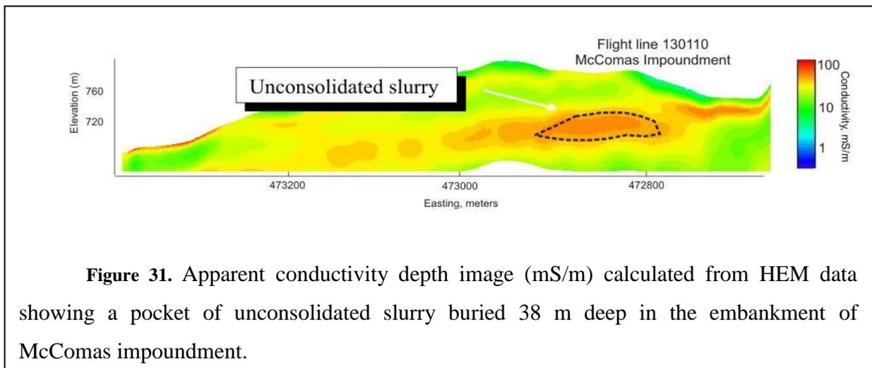
**Figure 31.** Apparent conductivity depth image (mS/m) calculated from HEM data showing a pocket of unconsolidated slurry buried 38 m deep in the embankment of McComas impoundment.
