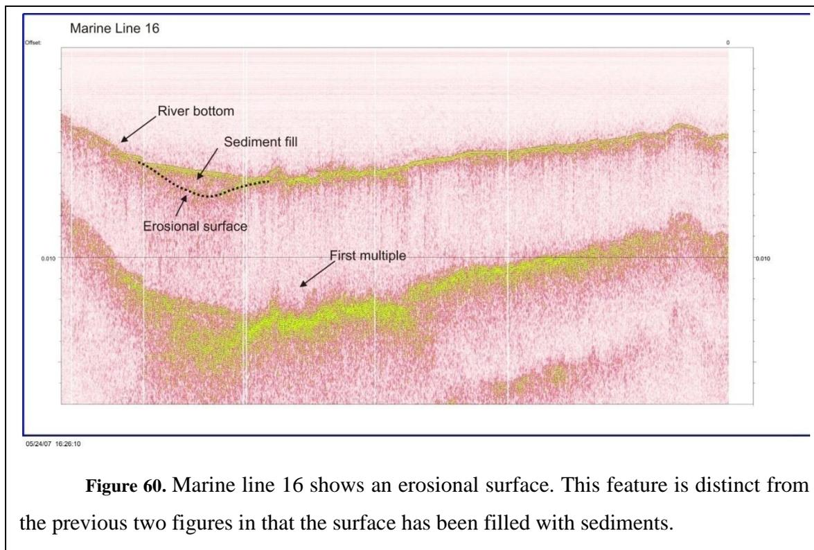
**Figure 60.** Marine line 16 shows an erosional surface. This feature is distinct from the previous two figures in that the surface has been filled with sediments.
