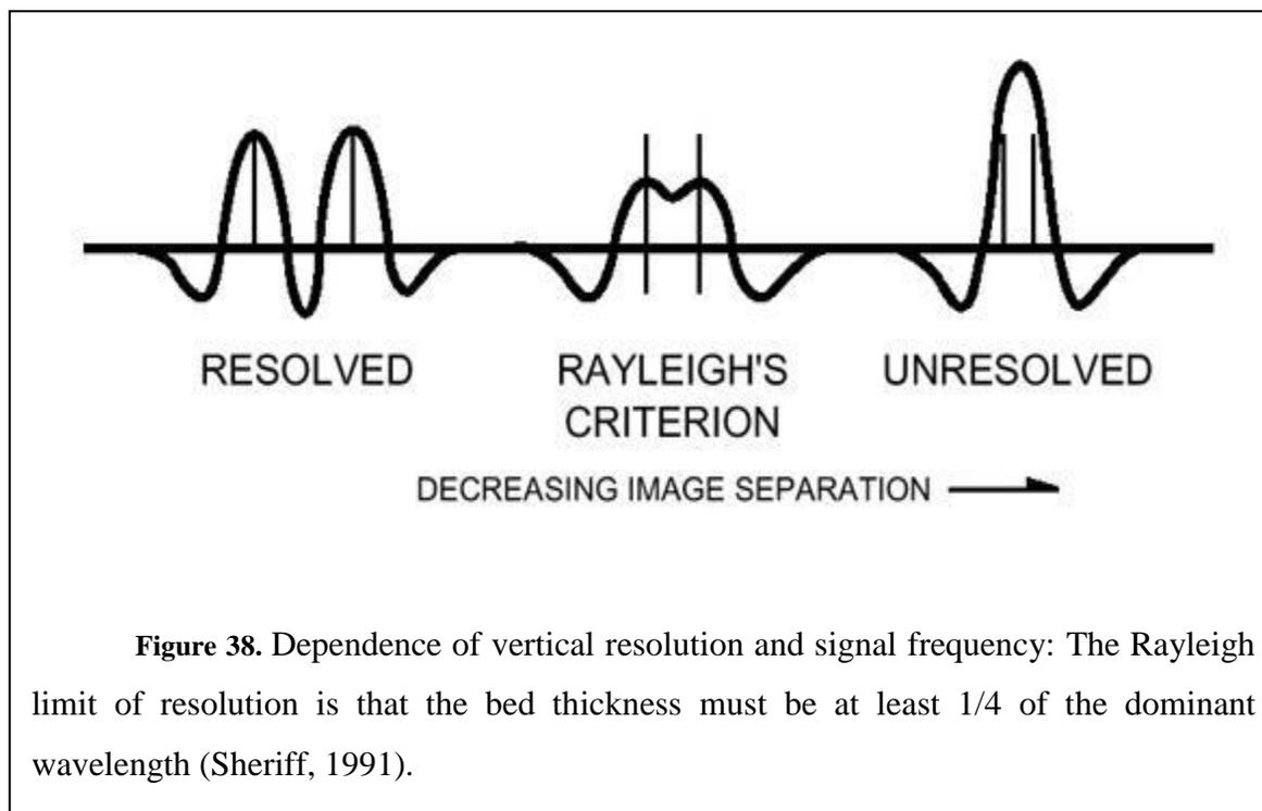
**Figure 38.** Dependence of vertical resolution and signal frequency: The Rayleigh limit of resolution is that the bed thickness must be at least 1/4 of the dominant wavelength (Sheriff, 1991).
