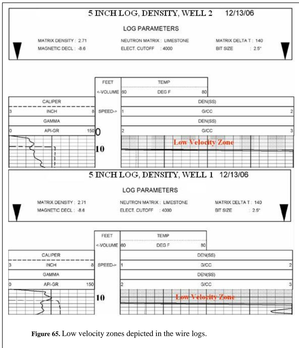
**Figure 65.** Low velocity zones depicted in the wire logs.
