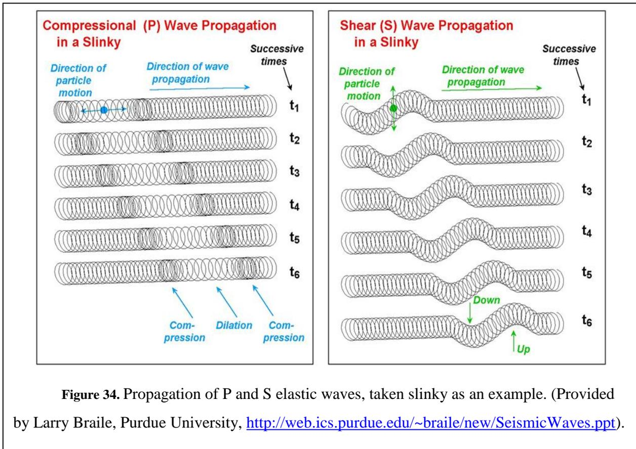
Figure 34. Propagation of P and S elastic waves, taken slinky as an example. (Provided by Larry Braile, Purdue University, <http://web.ics.purdue.edu/~braile/new/SeismicWaves.ppt>).
