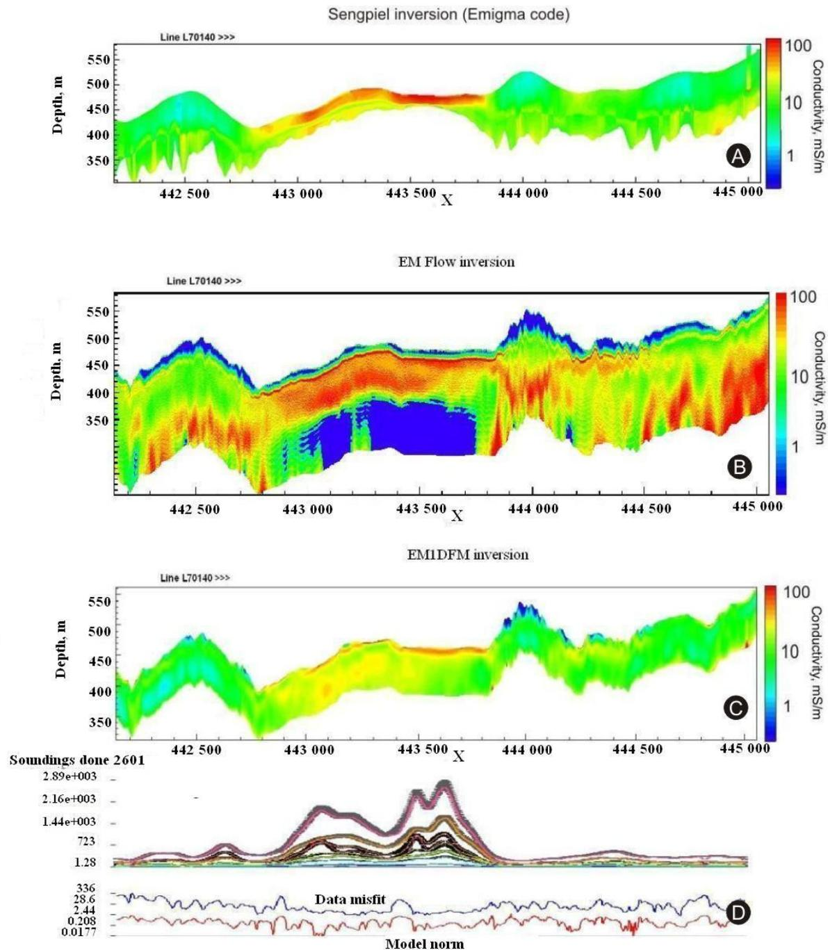
**Figure 18.** Conductivity depth images derived from three different inversion algorithms applied to flight line 70140. (A): Sengpiel technique. (B): EM Flow algorithm. (C): EM1DFM inversion with stabilization functional. (D): Data misfit and model norm for EM1DFM inversion are plotted for each observation point.
