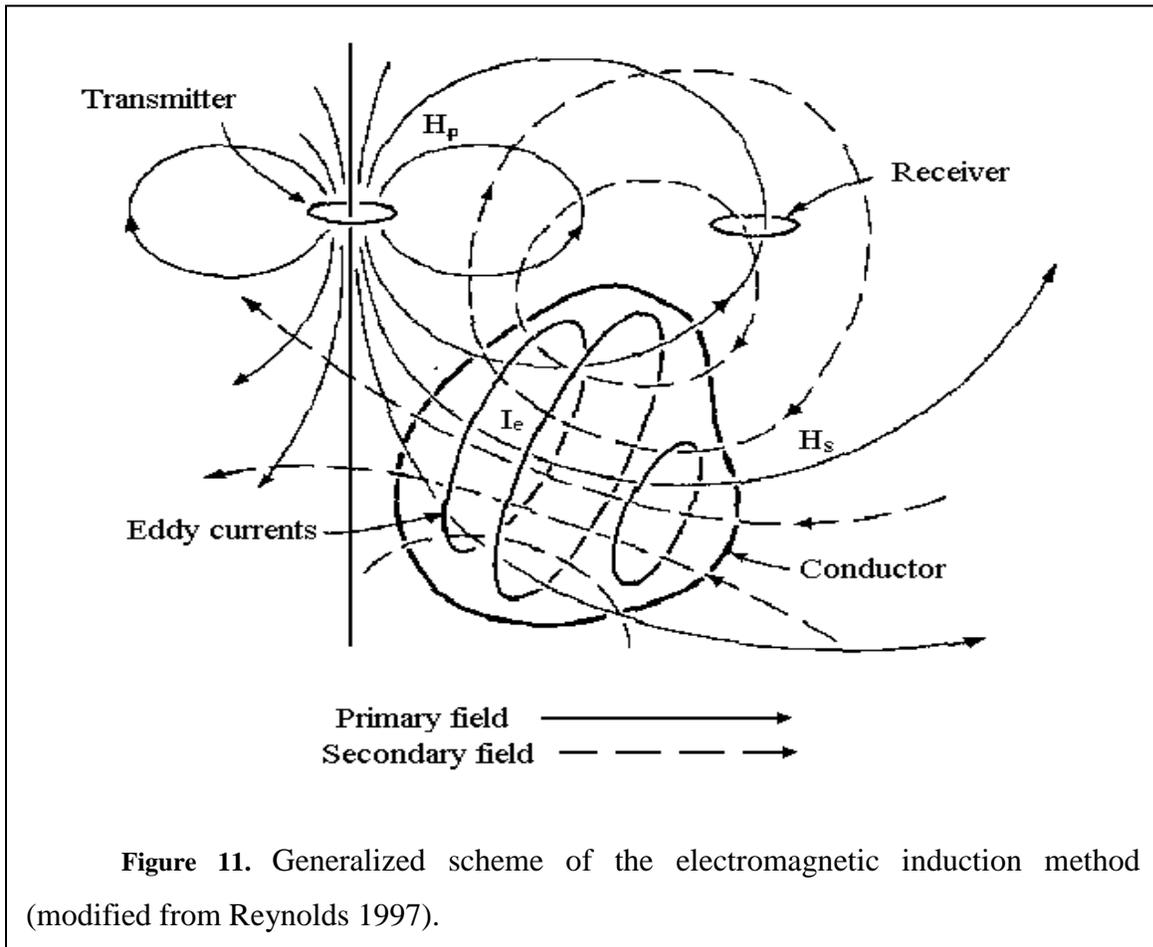
As it can be noted from Euler’s form of EM field propagation, the field can be presented as a combination of real (inphase) and imaginary (quadrature) components, which in free-space are shifted in phase by  $90^\circ$  (Fraser, 1976; Fraser, 1978; Fraser, 1979; Yakubovsky and Lyahov, 1988; Sharma, 1996). Applying the second order time differential operator to
