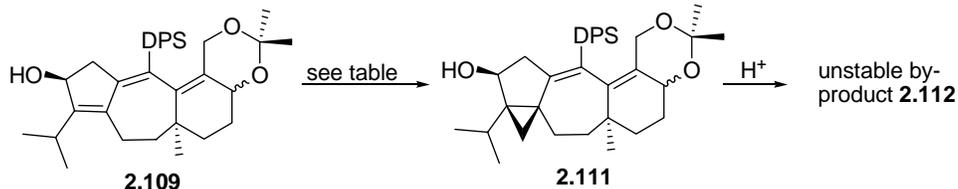
The reaction scheme shows the conversion of starting material **2.109** to product **2.111** using  $\text{Et}_2\text{Zn}$  and  $\text{I}_2\text{CH}_2$  (see table). Product **2.111** then reacts with  $\text{H}^+$  to form an unstable by-product **2.112**.
