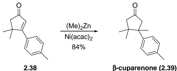
**Scheme 43.** An example of  $\text{Ni}(\text{acac})_2$  used as a catalyst for a conjugate addition reaction
