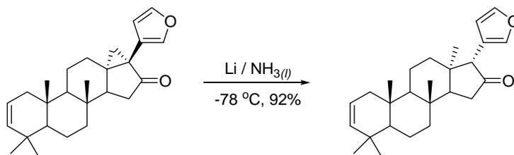
**Scheme 69.** Example of a reductive ring opening reaction of a cyclopropyl ketone
