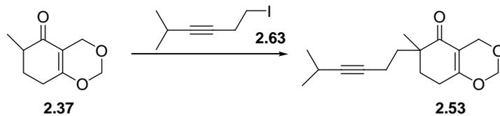
**7,8-Dihydro-6-methyl-6-(5-methylhex-3-ynyl)-4H-benzo[d][1,3]dioxin-5(6H)-one (2.53):** To a solution of LDA at -78 °C [prepared from diisopropylamine (0.17 mL, 1.2 mmol) in 1 mL of THF and *n*-butyllithium (0.70 mL of a 1.6 M hexanes solution, 1.1 mmol) at 0 °C for 30 min] was added a solution of enone **2.37** (0.13 g, 0.75 mmol) in 1.5 mL of THF dropwise via cannulation. After an additional 1.5 h at -78 °C, 1-iodo-5-methylhex-3-yne (**2.63**, 0.50 g, 2.2
