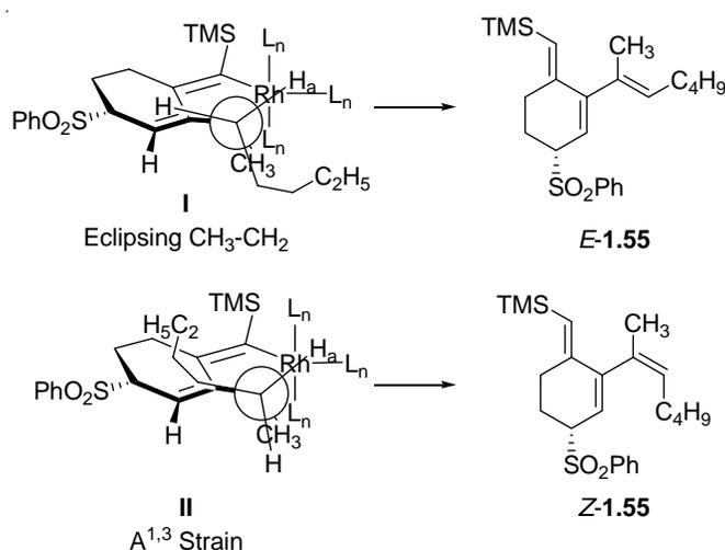
**Figure 5.** Explanation of *E/Z* selectivity in the Alder-ene reaction using allenyne **1.53**
