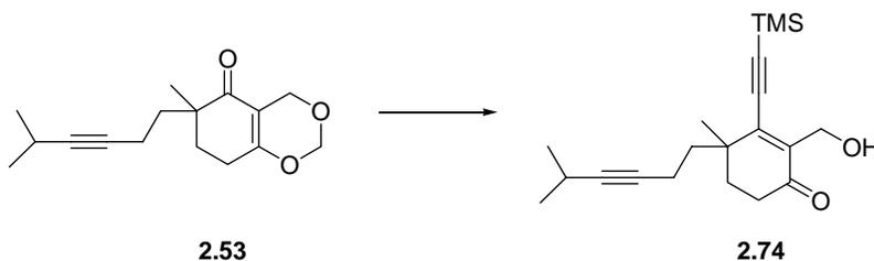
**2-(Hydroxymethyl)-4-methyl-4-(5-methylhex-3-ynyl)-3-(2-(trimethylsilyl)ethynyl)cyclohex-2-enone (2.74).** To a solution of trimethylsilylacetylene (2.1 g, 15 mmol) in 40 mL of THF at -78 °C was added n-butyllithium (8.4 mL of a 1.6 M hexanes solution, 14 mmol). After 1 h at -78 °C a solution of enone **2.53** (2.2 g, 8.4 mmol) in 40 mL of THF was added via cannulation. The reaction was allowed to warm to ambient temperature at which time the reaction was deemed
