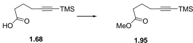
**6-Trimethylsilylhex-5-ynoic acid methyl ester 1.95.** To a solution of acid **1.68** (0.60 g, 3.3 mmol) in 2 mL of DMF was added  $\text{KHCO}_3$  (0.82 g, 8.2 mmol) and MeI (1.16 g, 8.15 mmol). The mixture changed from clear to yellow to orange/brown color and was left at ambient temperature. After 24 h complete consumption of starting material was seen by TLC, and the
