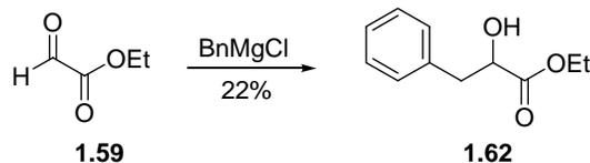
**Scheme 20. Addition of benzyl magnesium chloride to ethyl glyoxylate 1.59**
