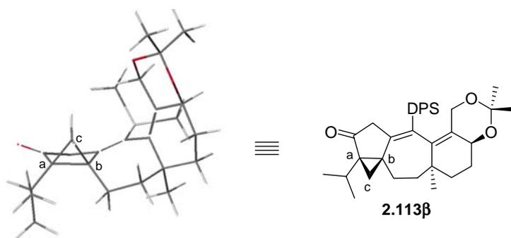
**Figure 34. Lowest energy conformation of 2.113 $\beta$  using Cache MM2; phenyl moiety removed after calculations for visual purposes**
