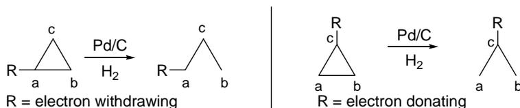
Figure 35. Selectivity of hydrogenation of substituted cyclopropanes
