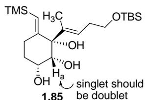
**Figure 14. Discrepancy in the  $^1\text{H}$  NMR of triol **1.85****
