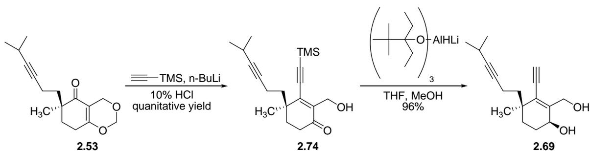
Scheme 58. Synthesis of diol **2.69** with correct stereochemistry
