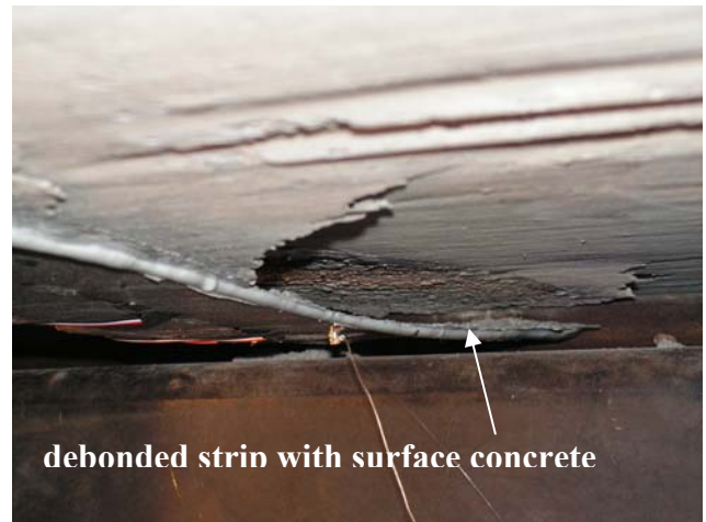
(b) Specimen 1x4 after testing
