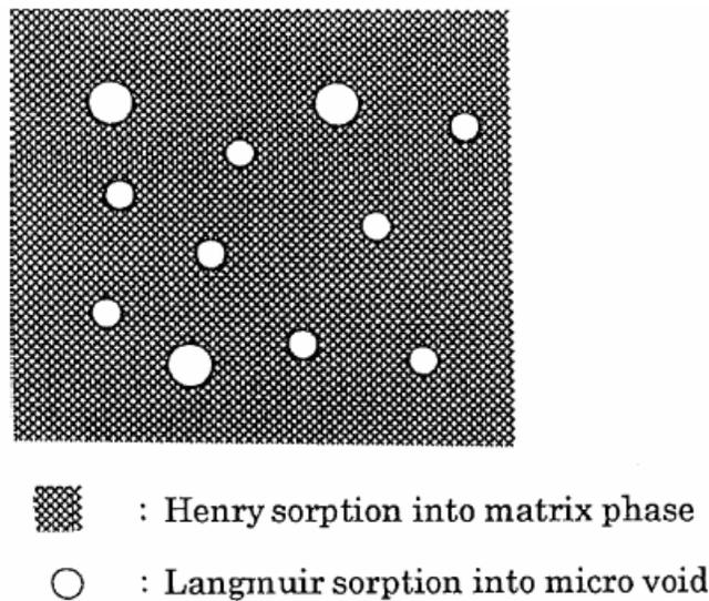
**Figure 2.** Schematic representation of polymeric glassy state depicting the matrix and microvoids
