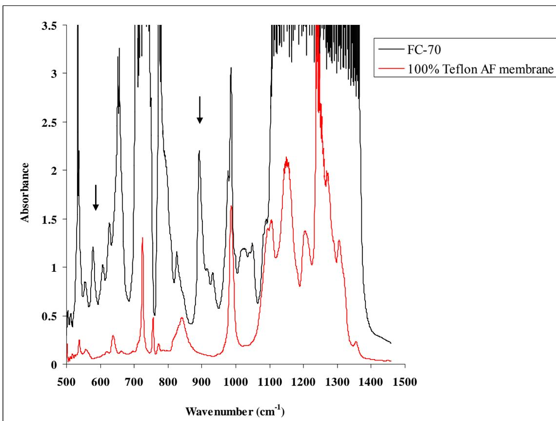
**Figure 11.** IR absorption spectra of 100% Teflon AF membrane and FC-70
