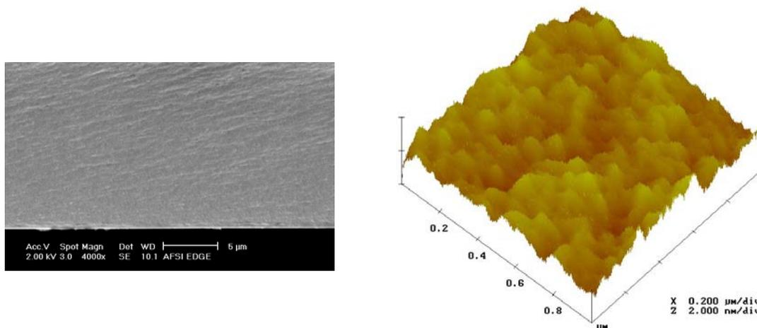
**Figure 5.** SEM image of the cross section of Teflon AF membrane (left); AFM image of the topography of Teflon AF membrane (right)<sup>1</sup>
