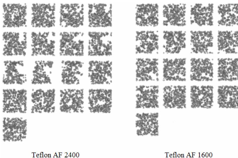
**Figure 8.** Qualitative “visual” impression of the free volume distributions for typical packing models of Teflons AF. The figures present a series of approximately monatomic layers cut perpendicular to the respective z-axis with the distance between successive slices of about  $3\text{\AA}$ .<sup>16</sup>
