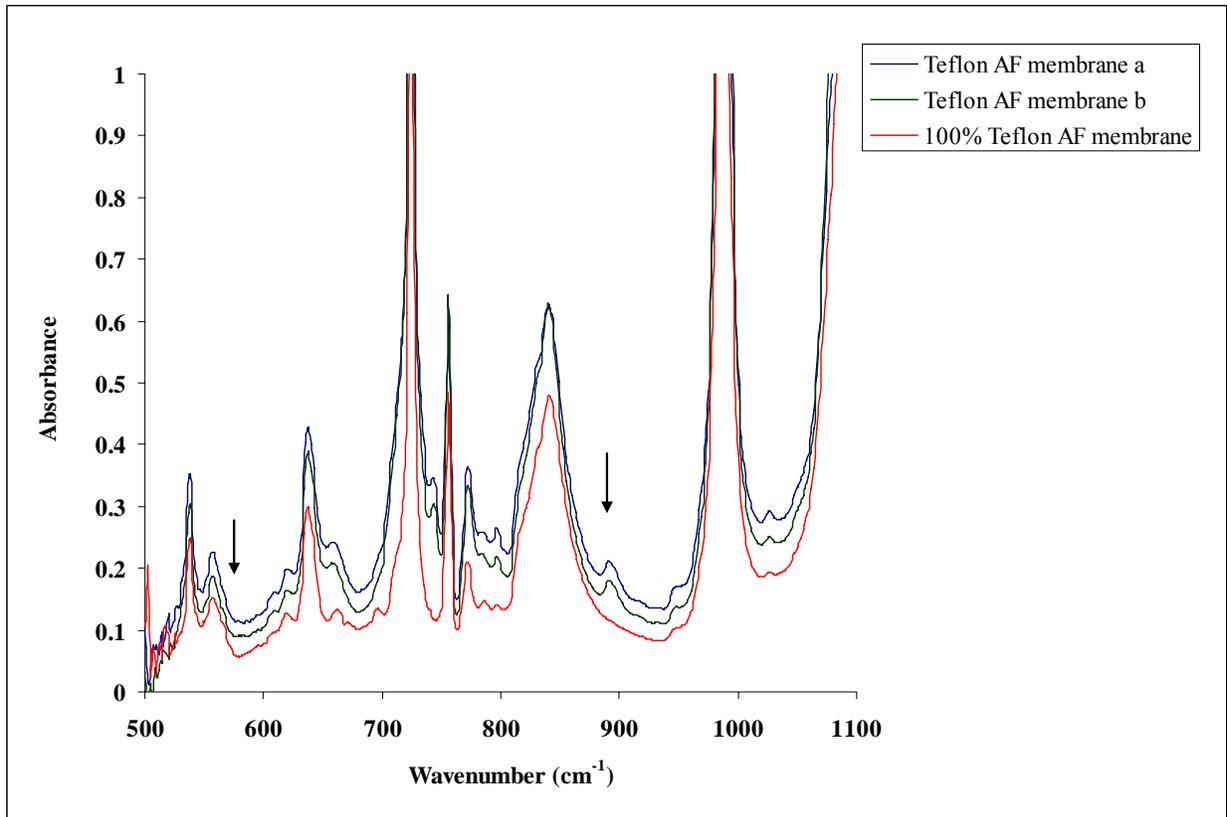
**Figure 12.** IR absorption spectra of Teflon AF membranes with and without FC-70
