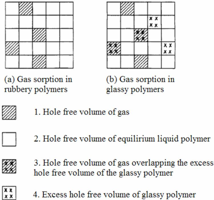
**Figure 3.** Schematic representation of the free volume based lattice. (a) represents gas sorption in rubbery polymers where two distinct sites can be identified. (b) represents gas sorption in glassy polymers where four distinct sites can be identified.<sup>48</sup>
