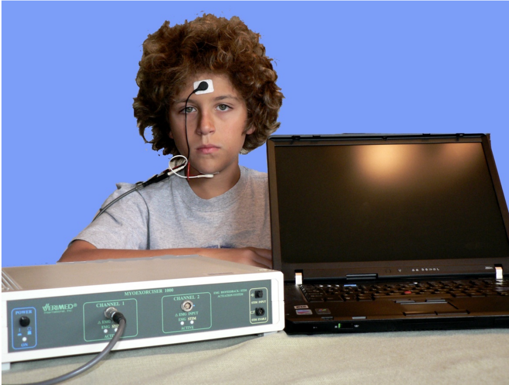
Figure 6. Instrumentation and Electrode Placement
