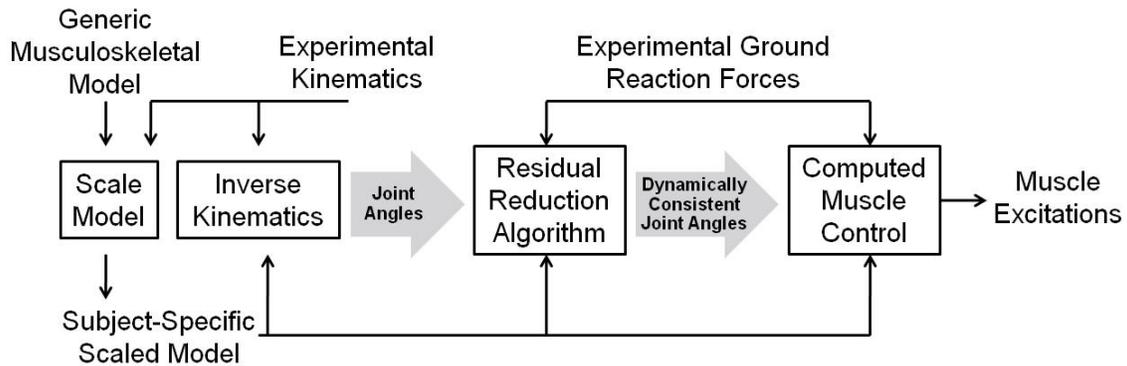
**Figure 6:** Steps for generating muscle excitations. A musculoskeletal model, experimental kinematics, and experimental ground reaction forces were inputted into OpenSim. Experimental kinematics were used to scale the generic musculoskeletal model. Model joint angles were found using an inverse kinematics approach. A residual reduction algorithm was used to refine the model kinematics. Muscle excitations were generated using a computed muscle control algorithm (Delp *et al.* 2007).
