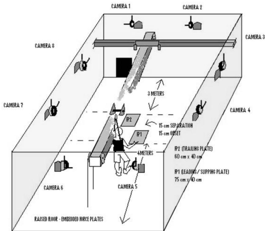
**Figure 3:** Schematic gait path layout. Vicon motion capture cameras are shown. Rectangles represent embedded force plates. Trolley and harness system are also shown.
